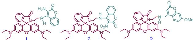
Scheme 1 Molecular structures for **L** as well as for two model reagents **2** and **R**.
