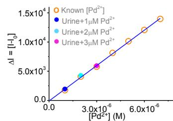
Fig 3. Plot of ΔI (I<sub>0</sub> - I) vs. [Pd<sup>2+</sup>], where I<sub>0</sub> and I are emission intensities of receptor **L** at 594 nm (λ<sub>ext</sub> = 530 nm) in the absence and presence of known [Pd<sup>2+</sup>] and urine sample spiked with a known [Pd<sup>2+</sup>].
