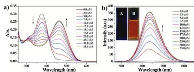
**Fig. 1** a) Absorption and b) fluorescence spectra ( $\lambda_{\text{ex}} = 460$  nm) of the  $\text{CHCl}_3$  solution of **1** ( $10.0 \mu\text{M}$ ) in the presence of HCl (from 0 to  $35.0 \mu\text{M}$ ); inset of Figure 1b shows photos of the solution of **1** ( $10.0 \mu\text{M}$ ) before (A) and after (B) addition of  $35.0 \mu\text{M}$  of HCl under 460 nm light irradiation.
