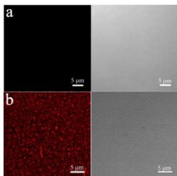
**Fig. 3** Fluorescence confocal laser scanning images of **1** (3 mL, 10.0 μM) before (a) and after (b) gamma-ray radiation (dosage = 8.0 Gy); the scale bar represents 5.0 μm.
