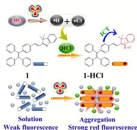
**Scheme 1.** Chemical structures of compound **1** and **1•HCl** and design rationale for the fluorescence turn-on detection of gamma-ray radiation.
