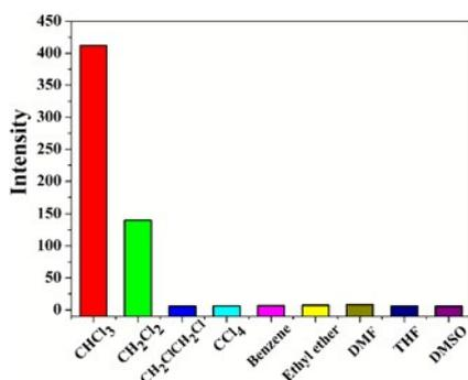
**Fig. 4** Variation of fluorescence intensity of **1** (10.0 μM) at 640 nm in different organic solvents after gamma-ray irradiation (dosage = 9.0 Gy); the excitation wavelength was 460 nm, and the concentration of **1** was 10.0 μM in CHCl<sub>3</sub>, CH<sub>2</sub>Cl<sub>2</sub>, 1, 2-dichloroethane, CCl<sub>4</sub> and 100.0 μM in benzene, ethyl ether, DMF, DMSO and THF.
