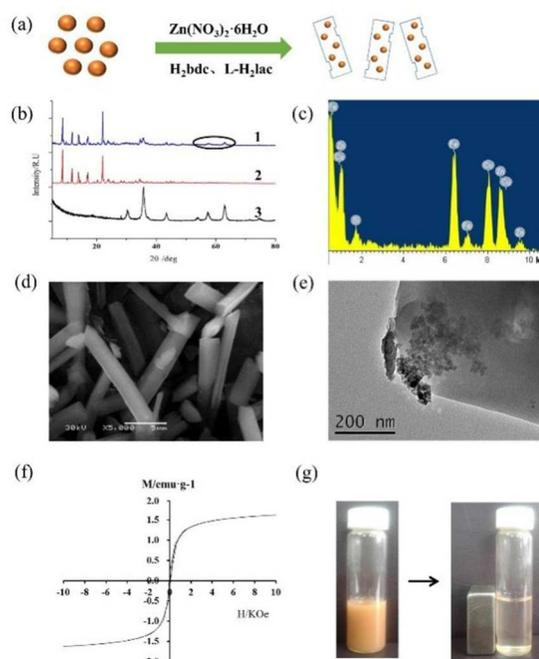
Figure 2. Synthesis and characterizations of  $Fe_3O_4@SiO_2$ -ZnBLD composites. (a) Schematic diagram of synthesis approach; (b) PXRD patterns of  $Fe_3O_4@SiO_2$ -ZnBLD (1), ZnBLD (2) and  $Fe_3O_4@SiO_2$  (3); (c) EDS result of  $Fe_3O_4@SiO_2$ -ZnBLD; (d) SEM image of  $Fe_3O_4@SiO_2$ -ZnBLD; (e) TEM image of  $Fe_3O_4@SiO_2$ -ZnBLD; (f) Magnetization curve of  $Fe_3O_4@SiO_2$ -ZnBLD; (g) Separation of  $Fe_3O_4@SiO_2$ -ZnBLD from solution under an external magnetic field.
