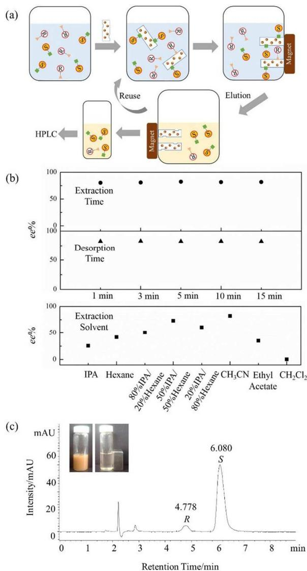
**Figure 3.** “Enantioselective fishing” process using  $\text{Fe}_3\text{O}_4@\text{SiO}_2\text{-ZnBLD}$ . (a) Schematic diagram; (b) Optimization of operation parameters; (c) Optimized result for methyl phenyl sulfoxide.
