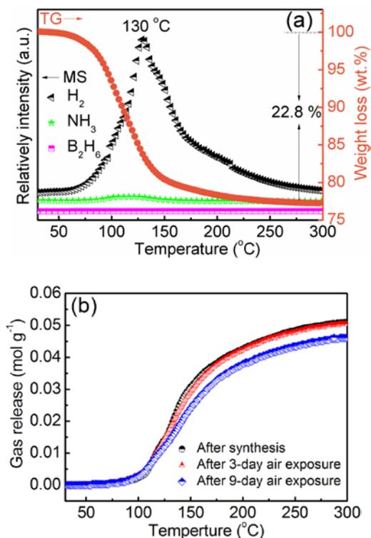
Fig. 2. (a) MS and TG profiles of Zr(BH<sub>4</sub>)<sub>4</sub>·8NH<sub>3</sub>; (b) TPD results for Zr(BH<sub>4</sub>)<sub>4</sub>·8NH<sub>3</sub>. All these measurements were performed with a heating rate of 5 °C min<sup>-1</sup> under an atmosphere of argon.
