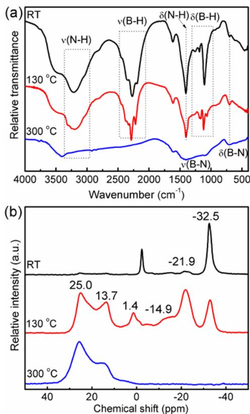
Fig. 3. (a) FT-IR spectra and (b)  $^{11}\text{B}$  NMR spectra for  $\text{Zr}(\text{BH}_4)_4 \cdot 8\text{NH}_3$  acquired at various temperatures.
