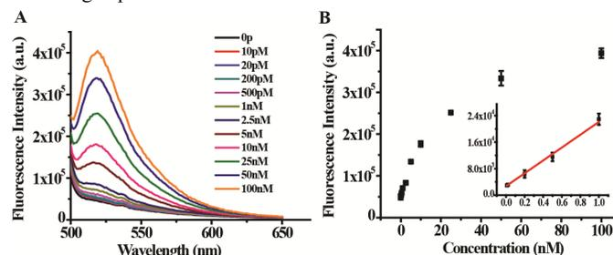
**Figure 2.** (A) Fluorescence emission spectra of DNA probes with different concentrations of let-7a. (B) Plot of fluorescence intensity as a function of the concentration of let-7a.
