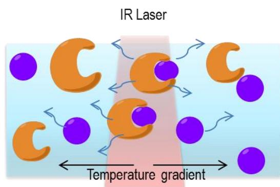
Figure 13. **Microscale thermophoresis (MST) is one of the latest methods to be applied to PPI evaluation.** The use of label-free off-surface techniques reduces the risk of inadequate evaluation caused by chemical modifications of the protein.
