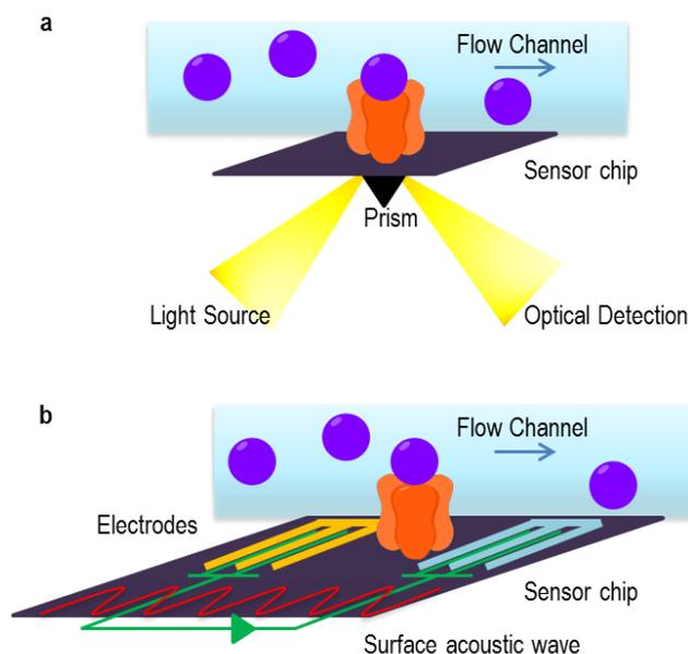
Figure 12. Label-free on-surface methodologies are often used in the first step of binder validation. Surface Plasmon Resonance (SPR) technique (a). Surface acoustic wave (SAW) technique (b).
