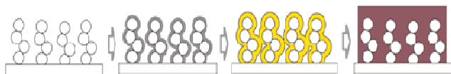
Scheme 1. Formation processes of the perovskite. on the mesoporous \text{TiO}_2 film, from electrodeposited PbO to \text{PbI}_2 , then \text{CH}_3\text{NH}_3\text{PbI}_3 .
