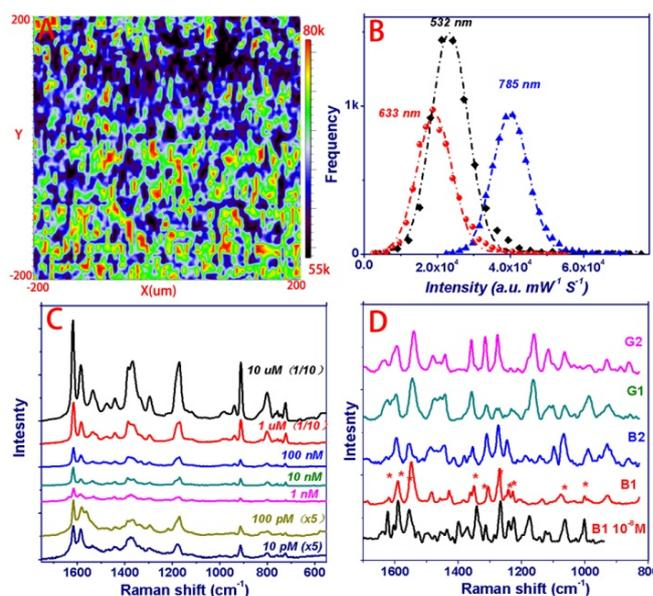
**Fig. 2** (A, B) SERS mapping at  $1077 \text{ cm}^{-1}$  excited at 785 nm and intensity distribution under different excitation wavelengths. (C) Representative SERS spectra of CV at various concentrations, and (D) SERS spectra of  $10^{-6}$  M AFTs and  $10^{-8}$  M AFT B1.
