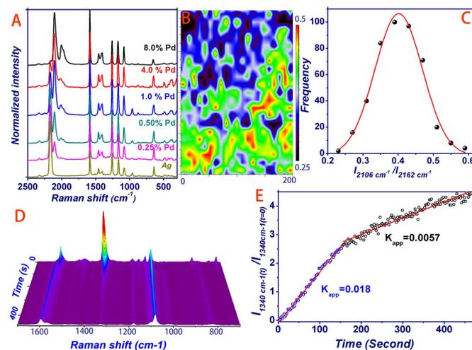
**Fig. 4** (A) Evolution of the SERS spectra of 2,6-DMPI with increasing amount of Pd; (B, C) Uniformity of Pd on Ag@Pd NPF as shown by SERS mapping; (D, E) 3D SERS mapping recorded on p-NTP-loaded Ag@Pd NPF (800 spectra, 0.5 s/spectrum), and calculation of the corresponding rate constant by a first-order reaction model.
