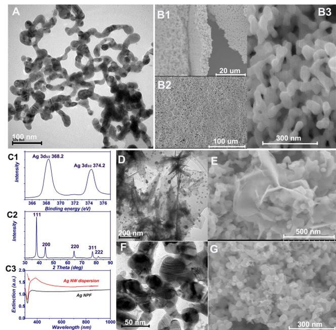
**Fig. 1** Morphological and spectroscopic characterization of fabricated nanostructures: (A) TEM images of Ag NWs; (B1-B3) FESEM image of Ag NPF at different magnifications; (C1-C3) XPS, XRD and UV-vis extinction spectra of Ag NWs and Ag NPF; TEM and FESEM image of Ag NPF- $\gamma$ -Fe<sub>2</sub>O<sub>3</sub> (D-E) and Ag@Pd NPF (F-G).
