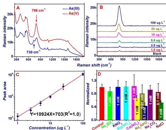
**Fig. 3** (A) SERS spectra of 10  $\mu$ g L<sup>-1</sup> As(III) and As(V) captured on Ag NPF- $\gamma$ -Fe<sub>2</sub>O<sub>3</sub> NSs; (B, C) background-subtracted SERS spectra of As(V) and the corresponding peak area as a function of concentration; (D) Tolerance of SERS detection of 7.5  $\mu$ g L<sup>-1</sup> or 0.1  $\mu$ M of As(V) to interference from co-existing ion on Ag NPF- $\gamma$ -Fe<sub>2</sub>O<sub>3</sub>.
