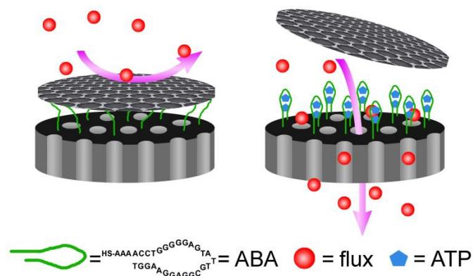
**Scheme 1** Schematic illustration of the graphene oxide-aptamer-nanochannel architecture and the principle for gating.
