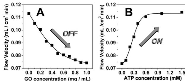
**Fig. 3** (A) Influence of the concentration of GO to the flow velocity. No ATP is presented here; and an OFF mode is launched under the coverage of GO. (B) Influence of the concentration of ATP to the flow velocity. After the ATP treatment, 1 mg/mL GO was adopted to cover the nanochannels.
