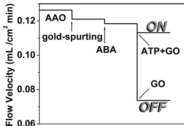
**Fig. 2** Flow velocity of water through the PAAOM during the whole gating process from gold-sputtering and ABA modification to ATP-controlled GO coverage. To accelerate the flow velocity, an extra pressure of 0.1 atm is added on the impouring side of PAAOM.
