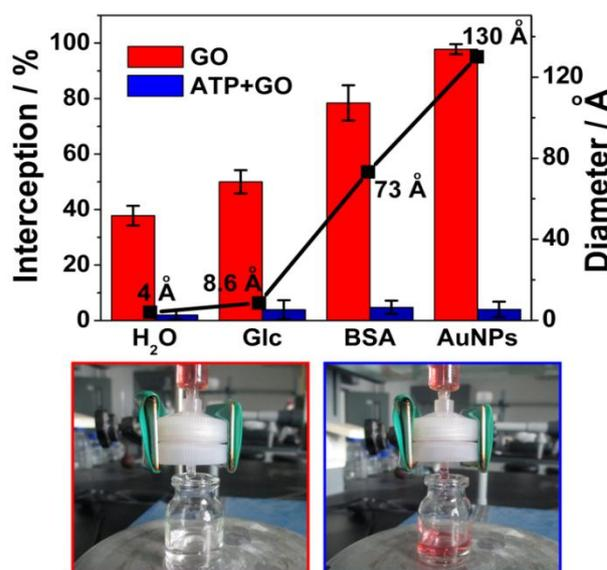
**Fig. 4** The interception towards different materials ( $H_2O$ , glucose, BSA and AuNPs) in ON (blue columns) and OFF (red columns) mode, respectively. In the case of  $H_2O$ , the flow velocity is involved for the calculation of the interception; while for the other three materials, the concentrations in the original solution and the effluent solution are measured. The bottom photos show the appearance of the gating results towards AuNPs in ON (right) and OFF (left) mode, respectively.
