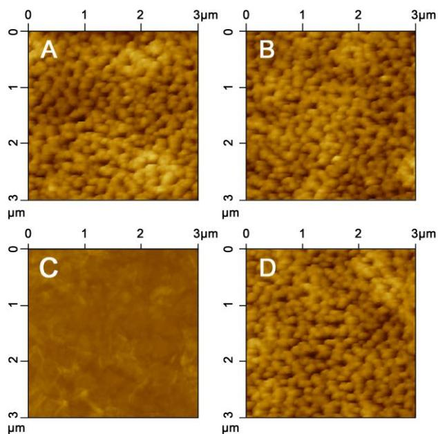
**Fig. 1** AFM images of PAAOM in different conditions. (A) gold-plated PAAOM (Au/PAAOM), (B) gold-plated and ABA-modified PAAOM (ABA/Au/PAAOM), (C) GO-covered PAAOM (GO/ABA/Au/PAAOM), and (D) ATP treated before the GO-coverage (GO/ATP-ABA/Au/PAAOM).
