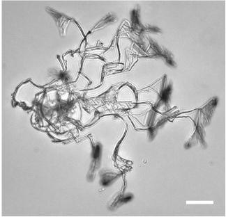
Fig. 4 Bright-field microscopic images of fluff-like water crystals in trans-DCE. Typical appearance of nucleating water crystals showing an asymmetric brush-like crystal growth in trans-DCE with 80 ppm water cooled to 213 K. Scale bar 50 μm.
