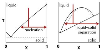
**Fig. 1** Liquid-solid phase diagrams for mixing two substances. (left) Two substances that mix well will exhibit a eutectic point. Cooling the mixtures will nucleate a solid phase. (**right**) Substances that mix poorly will give rise to liquid-liquid demixing on cooling. In particular cases, liquid-liquid demixing can be followed by crystallization of one of the phases.
