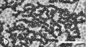
Fig. 3 Water crystal growth during liquid-liquid phase separation from trans-1,2-dichlorobenzene (trans-DCE). Different cooling rates result in different morphology of nucleating water crystals in trans-DCE with 458 ppm water. A cooling rate of 0.5 K/min (a) results in the formation of fluff-like wires at about 255 K while a rate of 50 K/min (b) results in round structures at about 233 K. Data taken as in Fig. 2. Scale bars 50  $\mu m$ .
