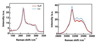
Fig. 6 Raman spectra of fluff-like water crystals. Confocal Raman microscopy experiments were performed using a Horiba LabRAM HR system. The excitation source was a 532-nm DPSS laser with a laser power at the sample stage of 28 mW. A 50 µm diameter aperture and 50× long-working distance objective were used to record the Raman spectra.
