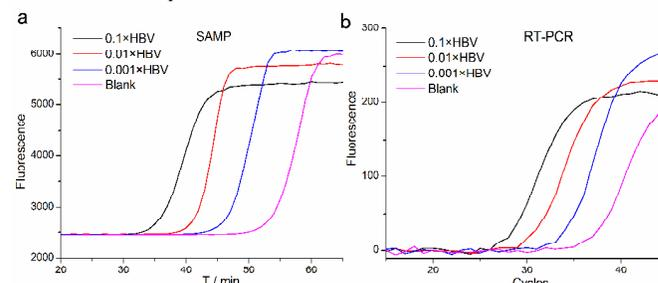
**Fig.3** SAMP and RT-PCR detection of HBV DNA. The RT-PCR solution contained 1  $\mu$ L serially diluted HBV DNA, specific primer set (200 nM each), and 5  $\mu$ L of SsoAdvance™ SYBR Green Supermix in a final volume 10  $\mu$ L. The RT-PCR was carried out as previously reported<sup>26</sup>.
