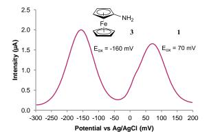
Fig. 1 Differential pulse voltammogram obtained for substrate 1 (100 μM) and ferrocenylamine 3 (100 μM) in 0.05 M pH 9 Tris buffer.
