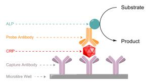
Scheme 3 An illustration of the ELISA format for CRP immunoassay used. Electrochemical detection obtained using DPV with either 1 or AA2P as the substrate.
