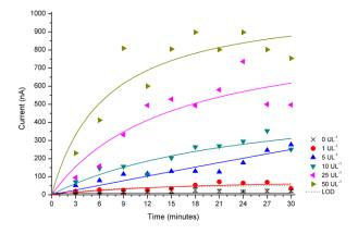
Fig. 5 Amperometric response of ferrocenylamine released from substrate 1 (50 μM) after the addition of ALP in different concentrations. Error bars indicate standard deviations (n = 3). LOD calculated as  $3 \times$  standard deviations higher than the mean.
