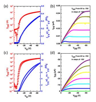
Fig. 4 Transfer and output characteristics of DAP1 (a, b) and DAP2 (c, d) devices with ODTS treatment.
