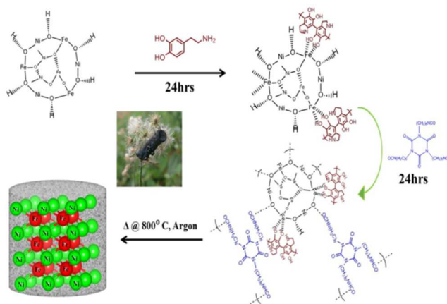
Figure 3: Schematic representation of Ni-Fe monolith synthesis (Photograph of Ni-Fe/C monolithic piece resting on dandelion flower parachute ball is given to show its light-weight)
