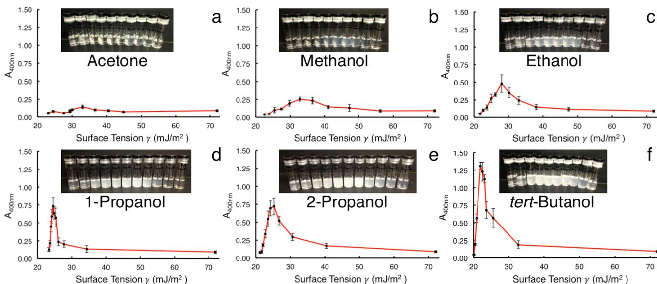
**Fig. 1** UV-vis data for BNNS in different co-solvent systems. Absorbance values were recorded at 400 nm; all data were averaged over five trials. From left to right, both the vials and the data points represent 100, 90, 80, 70, 60, 50, 40, 30, 20, 10, and 0 w/w% solvent in water. There are 11 vials present for both 1-prop (d) and IPA (e) to include 0 w/w% solvent (pure water), which can be seen as the rightmost vial in each photo.
