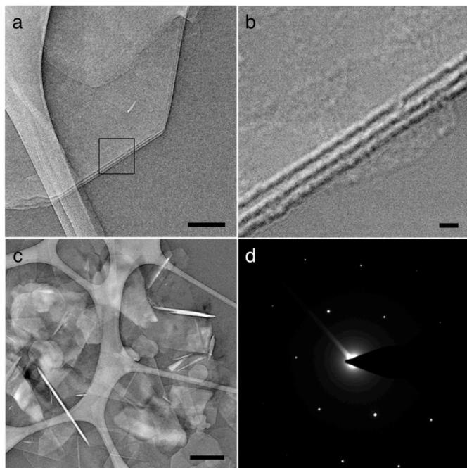
**Fig. 3** TEM micrographs of BNNS after sonication for 3 hr in 60% tBA. a) A few-layered BNNS sample. A carbon support can be seen through the exfoliated sheet. b) The magnified image of the square outline from Fig. 3a. c) Evidence for scrolling of the BNNS. The bright white “lines” are where the sheets have scrolled. d) Diffraction pattern of a few-layered BNNS. Scale bars represent a) 100 nm, b) 10 nm, and c) 0.5  $\mu\text{m}$ .
