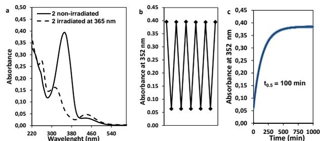
Fig. 3 UV-vis absorption spectra of *trans*- and *cis*-**2** ( $20 \times 10^{-6}$  M solution in MeOH) (a). Switching cycle of **2** (b). Kinetic study for the *cis* - *trans* isomerisation. Blue line represents the measured changes in absorbance, black line represents the fitting with single exponential decay (c).
