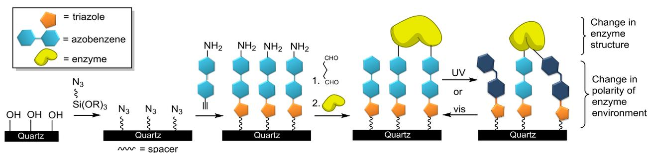
Fig. 1 Immobilisation of lipase on a quartz surface through a photoswitchable linker.
