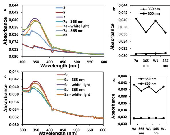
**Fig 5** UV-vis absorption spectra of clean quartz surface **3**, azide-bearing surface **5**, azobenzene-modified surface **7** and glutaraldehyde-modified surface **8a** (a). The switching cycle of **7** (b). UV-vis absorption spectra of lipase-modified surface **9a** (c). The switching cycle of **9**(d).
