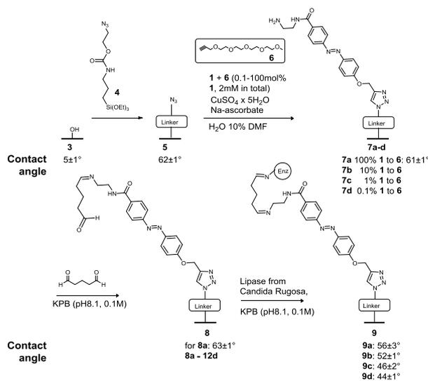
Fig. 4 Immobilisation of lipase from *Candida Rugosa* through the photoswitchable linker **1**. a-d indicate the mol% of **1** (100-0.1) with respect to **6** in the mixture.
