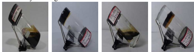
Fig. 4 (a) A sample of crude oil before gelation (b) A gelled sample of crude oil and D-1 at 0.5% (w/v) concentration (c) A biphasic system of saline water and crude oil before addition of the gelator (d) The biphasic system of water and crude oil after gelation of the crude oil with D-1.
