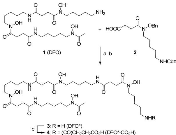
Scheme 1. Synthesis of DFO\* and its BFCA-analogue. a) HATU, DIPEA, DMF, rt; b) 10% Pd/C, H<sub>2</sub> (1 bar), MeOH, rt; c) succinic anhydride, NEt<sub>3</sub>, DMF, rt.
