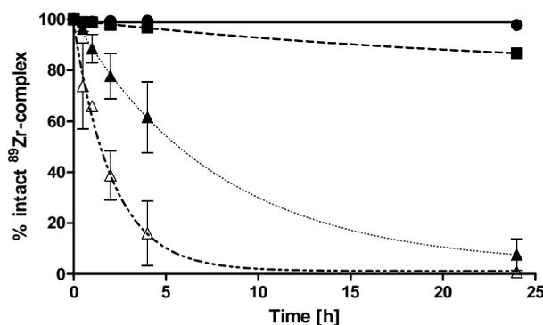
Figure 2. Stability of <sup>89</sup>Zr-complexes in DFO challenging experiments. (●): <sup>89</sup>Zr-**5**, 300-fold excess DFO; (▲): <sup>89</sup>Zr-**6**, 300-fold excess DFO; (■): <sup>89</sup>Zr-**5**, 3000-fold excess DFO; (Δ): <sup>89</sup>Zr-**6**, 3000-fold excess DFO (n= 2-3, presented as mean ± SD).
