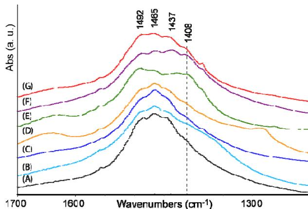
**Fig. 3** FTIR spectrum in the range of  $\nu_3$  band of: (A) vat1; (B) vat2; (C) vat1-pAsp; (D) vat2-pAsp; (E) *H. momus* spicule; (F) *C. nasus* asteriscus; (G) lackluster pearl. The full spectra in the range  $4000\text{--}500\text{ cm}^{-1}$  are reported in Fig. S2.
