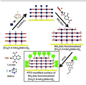
**Figure 22.** Assembly of a thin film of  $[Cu_2(1,4-ndc)_2(dabco)]_n$  on a gold surface, followed by addition of a monolayer of 2-NH<sub>2</sub>-1,4-bdc on the outer surface of the film, using a layer-by-layer deposition approach. The outer layer can then be further functionalized by post-synthetic modification, in this case, tagging FITC units to the reactive amino functions. Reprinted (adapted) with permission from Reference 75. Copyright (2011) American Chemical Society.
