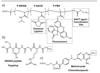
**Figure 9. a)** Chemical structure of the RAFT random co-polymer, comprised of *N*-isopropylacrylamide (NIPAM), *N*-acryloxysuccinimide (NAOS), and fluorescein-*O*-methacrylate (FMA) monomers, used to coat  $[Gd(1,4-bdc)_{1.5}(H_2O)_2]_n$  nanoparticles. The activated NHS ester allows post-synthetic conjugation of **b)** targeting GRGDS peptides and **c)** methotrexate chemotherapeutic units through reaction with free amino groups.
