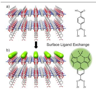
Figure 11. Schematic diagram to demonstrate the exchange of surface ligands from a) 1,4-benzenedicarboxylate units to b) fluorescent BODIPY linkers in  $[Zn_2(1,4-bdc)_2(dabco)]_n$ . Ligand exchange only occurs at the carboxylate terminated [100] surfaces of the MOF as a result of the functional group complementarity with the BODIPY ligand.
