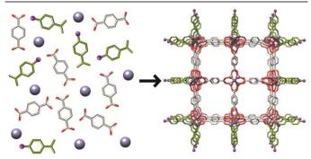
**Figure 2.** Schematic illustration of coordination modulation, where a monodentate ligand, or modulator, caps MOF crystal growth, using MOF-5 as an idealized example.
