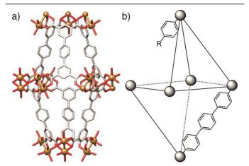
**Figure 5.** a) Section of the crystal structure of NOTT-101 (redrawn from CCDC deposition CESFOW). b) Simplified diagram to illustrate the introduction of defects within NOTT-101 when isophthalate modulators are incorporated into the synthesis of the MOF, generating mesopores with additional functional groups (labelled R).
