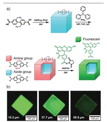
**Figure 17. a)** Synthetic scheme for surface functionalization of an azide substituted MOF through a size-selective, surface limited Staudinger reduction to amino groups, which are subsequently reacted with NHS-activated fluorescein tags. **b)** Confocal fluorescence microscopy shows the fluorescence, and so location, of the fluorescein units is confined to the surface of the MOF. Adapted from Reference 62 with permission from The Royal Society of Chemistry.
