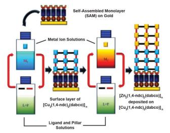
Figure 21. Mechanism for the preparation of an epitaxial MOF thin film [Zn<sub>2</sub>(1,4 $ndc)_2(dabco)]_n \quad deposited \quad on \quad [Cu_2(1,4-ndc)_2(dabco)]_n \quad in \quad a \quad layer-by-layer$ deposition approach on a self-assembled monolayer. Adapted from Reference 74 with permission from The Royal Society of Chemistry.
