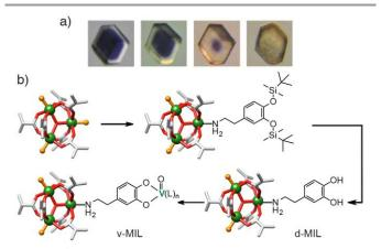
**Figure 13. a)** Photographs of metal cation exchange in  $[Co_6(1,3,5-btb)_4(4,4'-bipy)_3]_n$ , occurring from the surface of the crystal inwards. Reprinted (adapted) with permission from Reference 51. Copyright (2012) American Chemical Society. **b)** Scheme showing coordination of bulky TBDMS-protected dopamine to the  $Cr^{3+}$  cations of the SBUs at the surface of MIL-101(Cr) only, which can then be deprotected and vanadylated.
