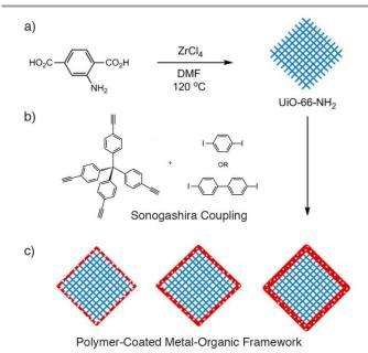
**Figure 10.** a) Synthesis of UiO-66-NH<sub>2</sub>, which can **b)** be coated with a microporous polymer through a Sonogashira reaction to yield **c)** MOF particles with polymer coatings of varying thicknesses, depending on reaction conditions. Reprinted (adapted) with permission from Reference 47. Copyright (2014) American Chemical Society.
