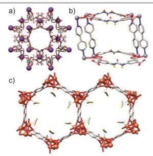
**Figure 1.** Sections of the solid-state structures of **a)** CD-MOF-2, whose surfeit of pendant hydroxyl units facilitates transient chemisorption of  $CO_2$ , **b)** NU-601, a urea functionalized MOF which acts as a heterogeneous organocatalyst, and **c)** iron dioxidoterephthalate, binding acetylene through interactions with coordinatively unsaturated  $Fe^{2+}$  cations. Redrawn from CSD depositions LAJLEP, HAPHUD and SARGID, in turn.
