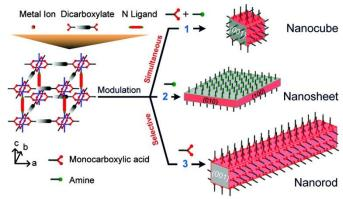
**Figure 6.** The effect on crystal shape of varying the ratios of face-selective carboxylic acid and amine modulators during the synthesis of pillared MOFs. Reprinted with permission from Reference 32. Copyright (2012) American Chemical Society.
