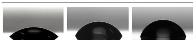
**Figure 3** Water droplets on amine-coated quartz (left), **MS1** (middle), and **MS2** (right). The measured water contact angles are 40°, 63° and 73°, respectively.
