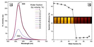
Fig. 2. Change in FL intensity (A) and  $\Phi_{\rm F}$  (B) of molecule 2 in THF/water mixtures with different  $f_{\rm w}$  values; the inset images show the corresponding FL photographs. Concentration: 10  $\mu$ M;  $\lambda_{\rm ex}$ : 365 nm.
