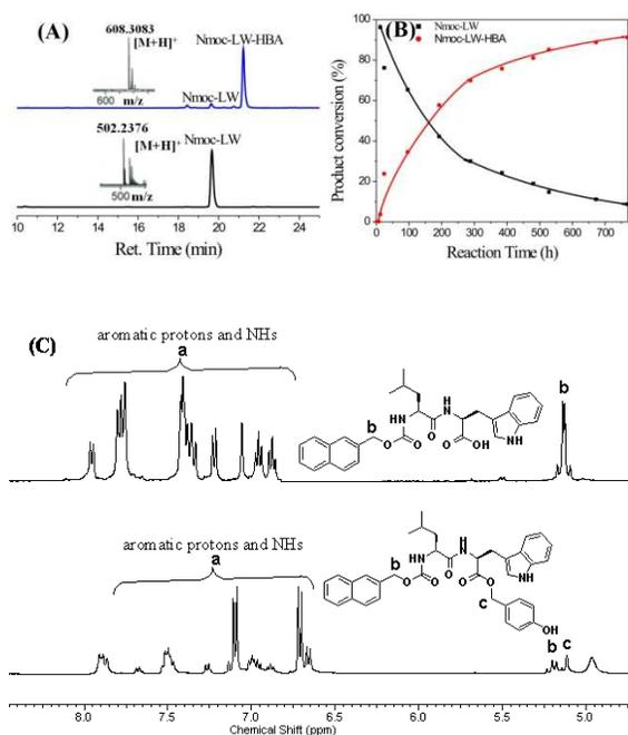
**Fig. 2** (A) HPLC trace analysis of enzyme catalyzed esterification of Nmoc-LW **1** to Nmoc-LW-HBA with its corresponding ESI-MS. (B) Real time HPLC analysis for the formation of Nmoc-LW-HBA. (C) Partial <sup>1</sup>H NMR of Nmoc-LW **1** and its corresponding dried Nmoc-LW-HBA hydrogel synthesized via CRL catalyzed esterification reaction in DMSO-d<sub>6</sub>.
