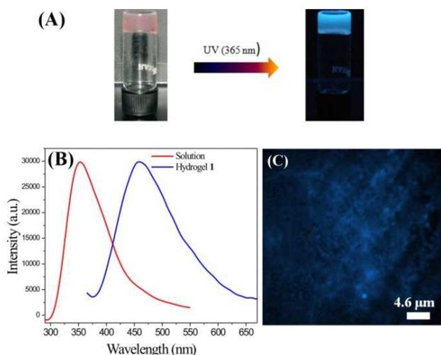
**Fig. 3** (A) Optical images of hydrogel Nmoc-LW-HBA **1** under daylight and under UV light (365 nm). (B) Normalized emission spectra of solution of Nmoc-LW **1** with HBA ( $\lambda_{\text{ex}} = 280$  nm) and hydrogel formed by Nmoc-LW-HBA ( $\lambda_{\text{ex}} = 365$  nm) and (C) fluorescence microscopy image of gel at 2 mmol L<sup>-1</sup> concentration.
