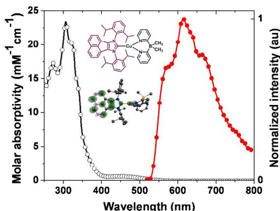
**Figure 4.** Absorption (room temperature,  $\text{CH}_2\text{Cl}_2$ ) and emission (77 K, 2-MeTHF) spectra of complex **4**. (inset) Molecular structure, optimized triplet geometry and spin density contour plot (isovalue:  $0.004 e a_0^{-3}$ ).
