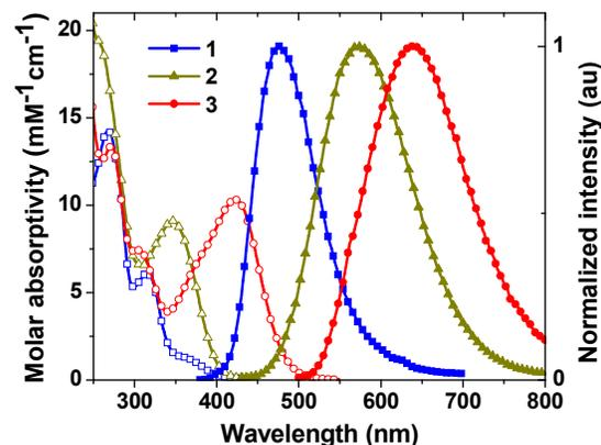
**Figure 2.** Absorption (open symbols, CH<sub>2</sub>Cl<sub>2</sub>) and emission (closed symbols, solid powder) spectra of complexes **1–3** at room temperature.
