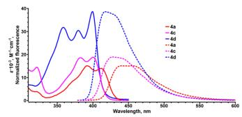
Figure 2. Absorption (solid) and emission (dashed) spectra of compounds **4a**, **4c** and **4d** in dichloromethane (DCM).
