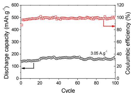
Fig. 5 Cycling performance of  $V_4O_7$  nanocross at high rate: (A) galvanostatic test of  $V_4O_7$  nanocross under  $3.05 \text{ A.g}^{-1}$ ; (B) corresponding discharge profiles of 100 cycles
