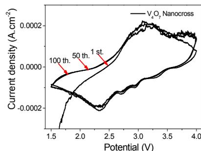
Fig. 4 CV test of V<sub>4</sub>O<sub>7</sub> nanocross under 0.5 mV.s<sup>-1</sup> current density.
