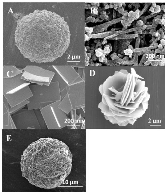
Fig. 1 Morphological characterization of VO<sub>x</sub> hierarchical structure with (A) 0 %, (B) 12.5 %, (c) 25%, (D) 75 % and (E) 95 % water content.
