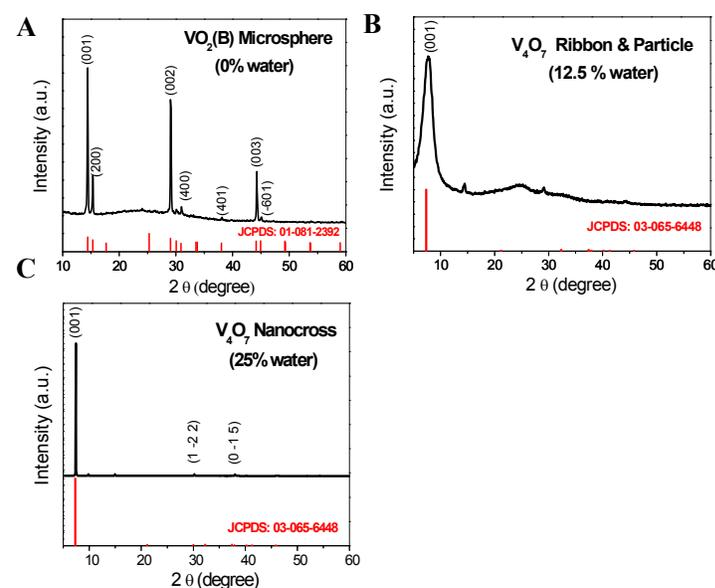
Fig. 2 Crystallinity characterization of VO<sub>x</sub> hierarchical structure with (A) 0 %, (B) 12.5 %, (c) 25% water content.
