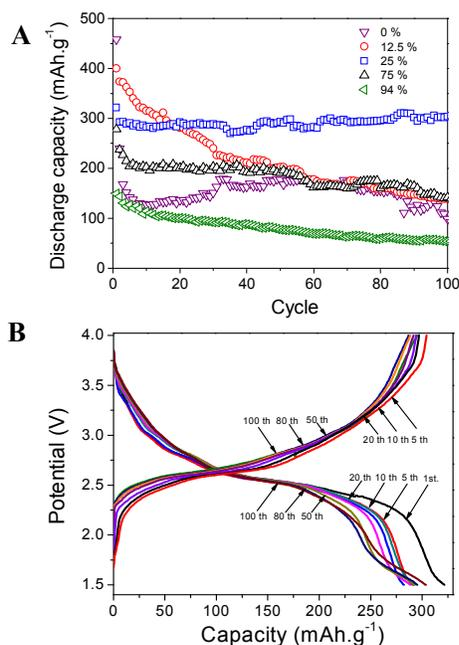
Fig. 3 Cycling performance of hierarchical VO<sub>x</sub> synthesized with different water content: (A) 100 cycles charge/discharge performance at 50 mA.g<sup>-1</sup>; (B) corresponding discharge profiles of 100 cycles of V<sub>4</sub>O<sub>7</sub> nanocross.
