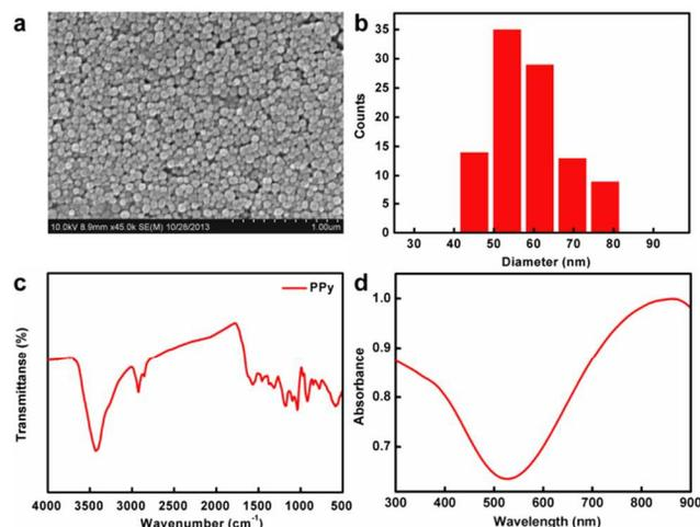
Fig. 1 The SEM image (a) and size distribution analysis (b) of PPy. The total number of PPy nanoparticles counted for the histogram was 100. (c) FTIR spectrum of PPy nanoparticles. (d) UV-vis-NIR absorbance spectrum of PPy nanoparticles.
