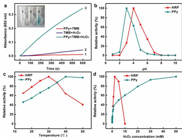
**Fig. 2** (a) Time-dependent absorbance changes at 652 nm of TMB in different reaction systems: (1) PPy + TMB, (2) TMB +  $\text{H}_2\text{O}_2$  and (3) PPy + TMB +  $\text{H}_2\text{O}_2$ . (b, c, d) The peroxidase-like activity of the PPy nanoparticles is dependent on pH (b) and temperature (c) and  $\text{H}_2\text{O}_2$  concentration (d).
