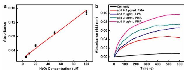
**Fig. 3** (a) H<sub>2</sub>O<sub>2</sub> concentration dependent UV absorbance containing the PPy/TMB kit. The background absorbance from the same solutions but without H<sub>2</sub>O<sub>2</sub> have been subtracted. Error bars represent standard deviation of three independent measurements. (b) Time-dependent absorbance changes at 652 nm of TMB from PBS solution containing PPy/TMB kit and RAW264.7 cells ( $3 \times 10^5$  cells) in the presence of different concentrations of PMA and LPS.
