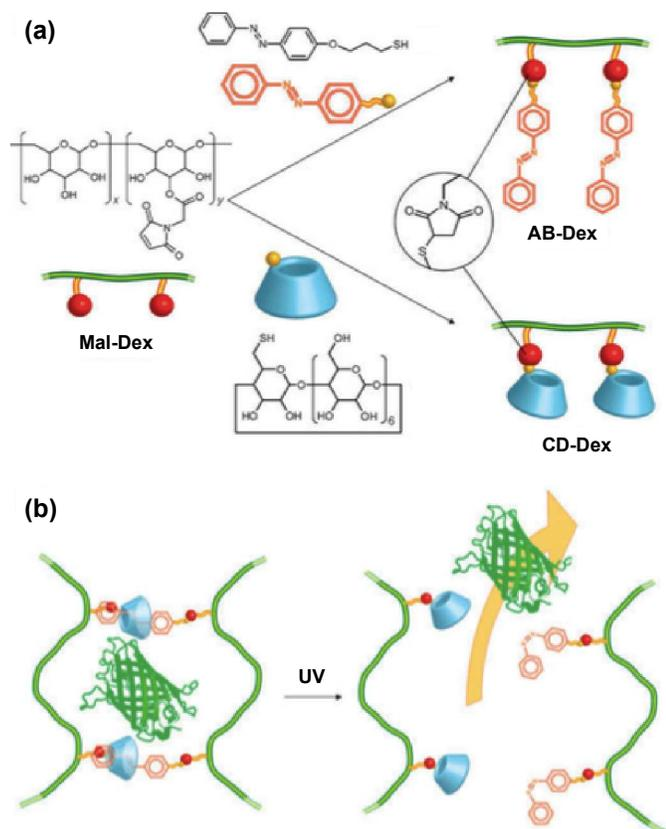
**Fig. 10** (a) Preparation of azobenzene-modified dextran (AB-Dex) and cyclodextrin-modified dextran (CD-Dex). (b) Photo-responsive protein release from the supramolecular hydrogels. Reproduced with permission from ref. 121. Copyright 2010, Royal Society of Chemistry.
