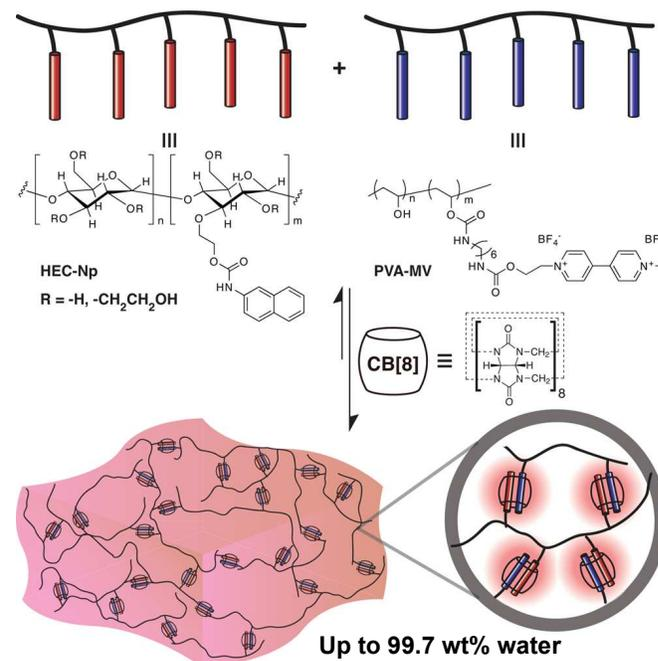
**Fig. 3** Schematic illustration of a supramolecular polymeric hydrogel formed through addition of CB[8] to a mixture of a naphthyl-functionalized cellulose (HEC-Np) and a methyl viologen-functionalized poly(vinyl alcohol) (PVA-MV) in water. Reproduced with permission from ref. 57. Copyright 2012, American Chemical Society.
