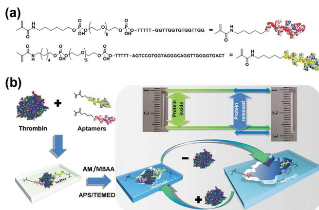
**Fig. 8** (a) Two different aptamers modified with a polymerizable methacrylamide terminus linked to the aptamer via a linker incorporating five thymidine units, six ethylene oxide units, and six methylene units. (b) Scheme of the biomolecular imprinting used to produce superaptamer thrombin-responsive hydrogels along with macroscopic volume change. Reproduced with permission from ref. 97. Copyright 2013, American Chemical Society.
