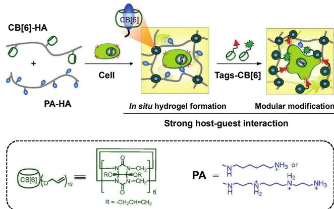
**Fig. 11** Schematic representations for *in situ* formation of supramolecular biocompatible hydrogel and its modular modification using highly selective and strong host-guest interactions. The simple mixing of CB[6]-HA and PA-HA in the presence of cells led to the formation of cell-entrapped supramolecular hydrogels, which was further modularly modified with various tags-CB[6]. Reproduced with permission from ref. 139. Copyright 2012, American Chemical Society.
