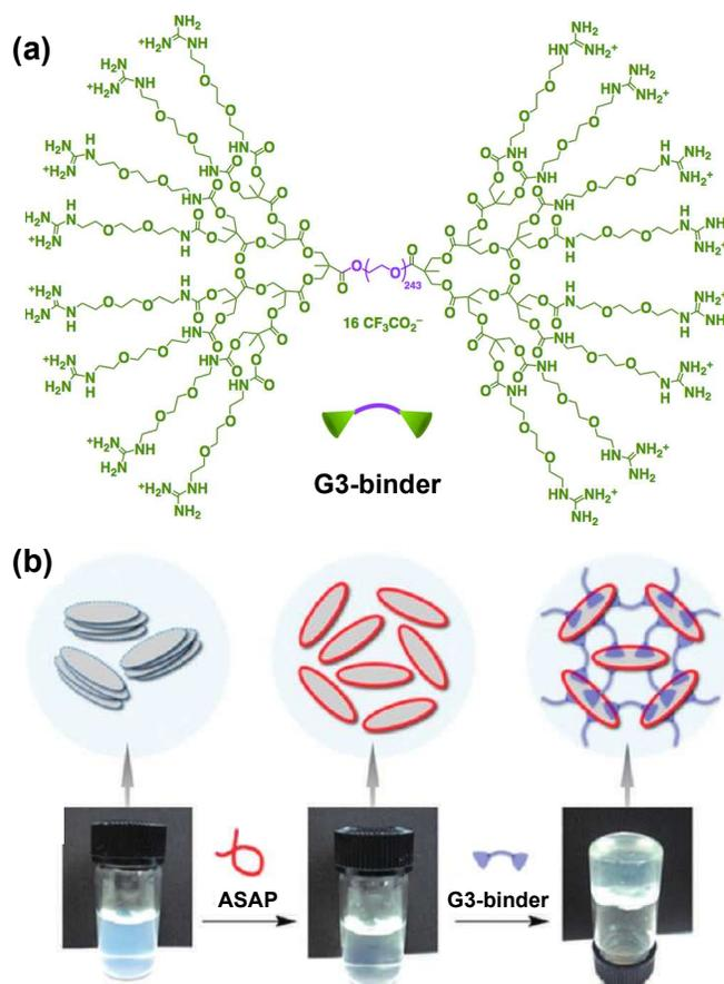
**Fig. 5** (a) Chemical structure of a G3 dendritic binder. (b) The preparation process of supramolecular hybrid hydrogels upon addition of a G3 dendritic binder into anionic sodium polyacrylate (ASAP) treated clay nanosheets in water. Photographs show the evolution of the systems upon addition of these components. Reproduced with permission from ref. 52. Copyright 2010, Nature Publishing Group.
