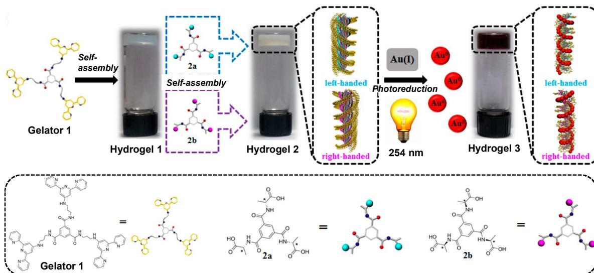
**Fig. 4** Schematic representation of the formation of supramolecular hybrid hydrogels resulting from controlled assembly of nanofibers with tunable helicity by addition of chiral **2a** or **2b** components, and further addition of Au(I) followed by UV exposure to produce helically templated gold nanoparticle superstructures. Reproduced with permission from ref. 54. Copyright 2014, American Chemical Society.
