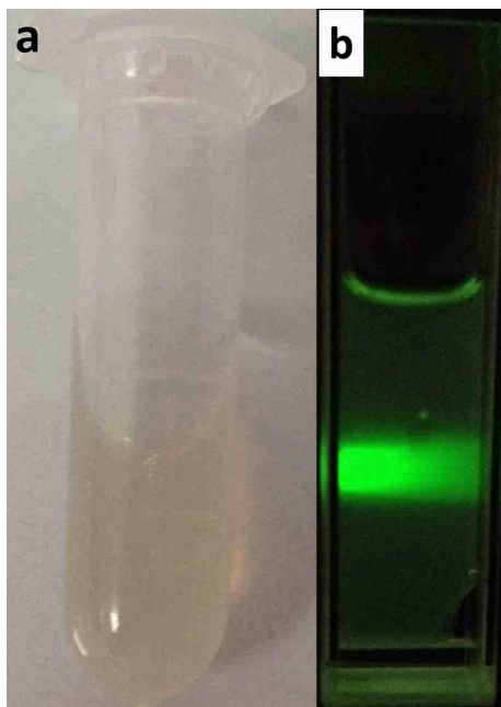
Fig. 9 The photographs of MNP-UCNPs suspension (a) and the luminescence of the suspension excited by a 980 \text{ nm} excitation laser (b)
