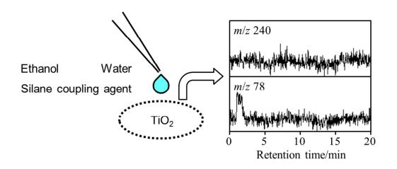
LI/TOFMS was applied to the measurement of pyrolysis products generated from silanized TiO<sub>2</sub> nanoparticles.
