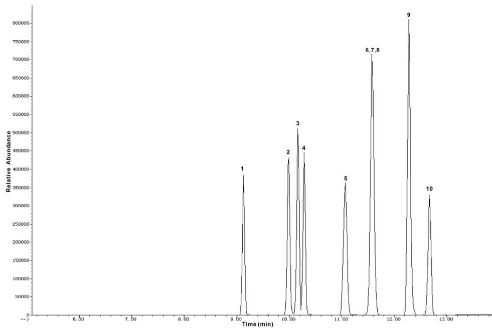
Fig. 3 The total ion chromatogram of the mixed standards and internal standards (I.S.).
