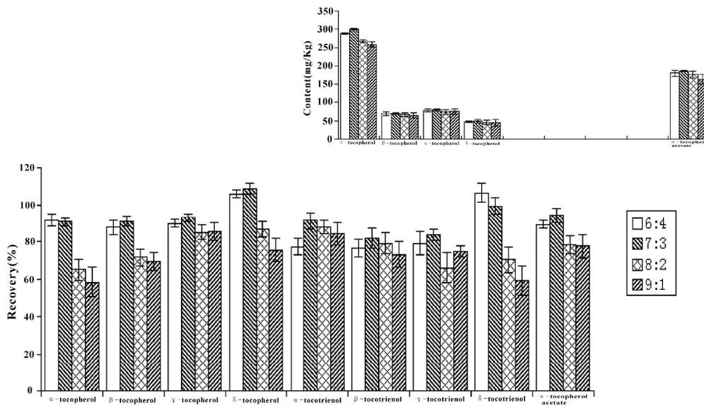
Fig. 2 Recoveries (below) and the detected content (above) of VE isomers using different proportion of methanol - hexane. (mean $\pm$ SD, n= 3).
