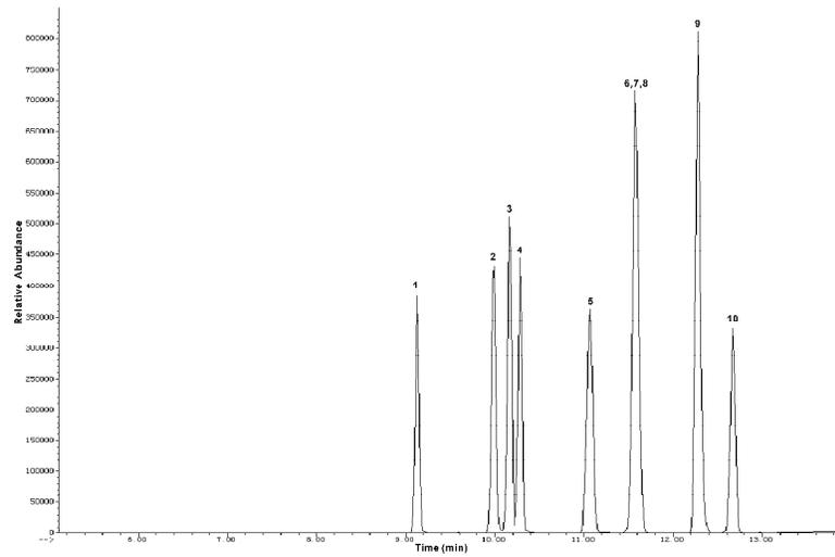
A gas chromatography-mass spectrometry (GC-MS) has been developed for the simultaneous determination of eight VE isomers and  $\alpha$ -tocopherol acetate in functional foods.
