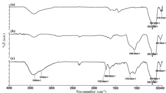
Fig. 3 FT-IR spectra of (a) MNPs, (b) SCMNPs and (c) VENMNPs
