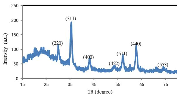
Fig. 4 XRD pattern for VENMNPs nanoparticles.
