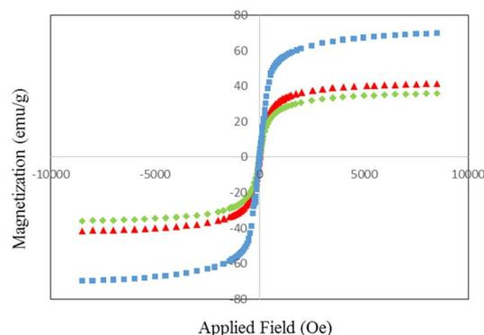
Fig. 6 Magnetization curves obtained by vibrating sample magnetometer (VSM) at room temperature: (■) bare MNPs; (▲) SCMNPs; and (●) VENMNPs nanoparticles.
