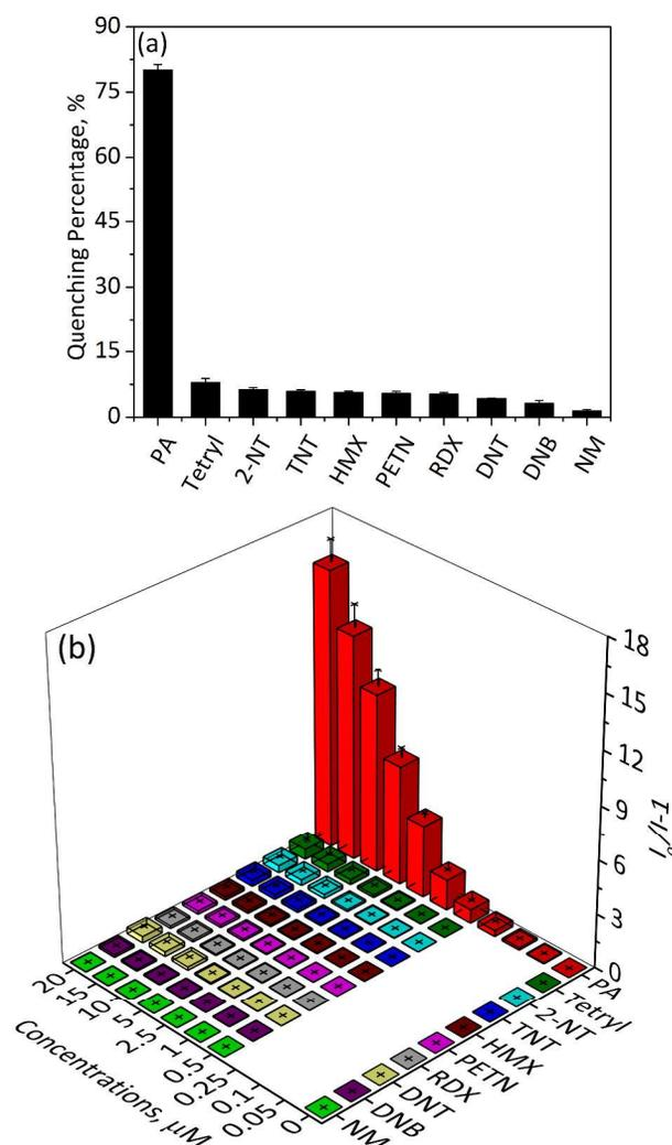
**Fig. 2** (a) Percentage of fluorescence quenching obtained for BSA fluorescent sensors upon addition of 2.5  $\mu\text{M}$  of different nitro-explosives (BSA concentration is 0.5  $\mu\text{M}$  BSA), indicating excellent selectivity for picric acid. (b) Stern-Volmer plots of BSA fluorescent sensors with different nitro-based explosives at 0.5  $\mu\text{M}$  BSA.
