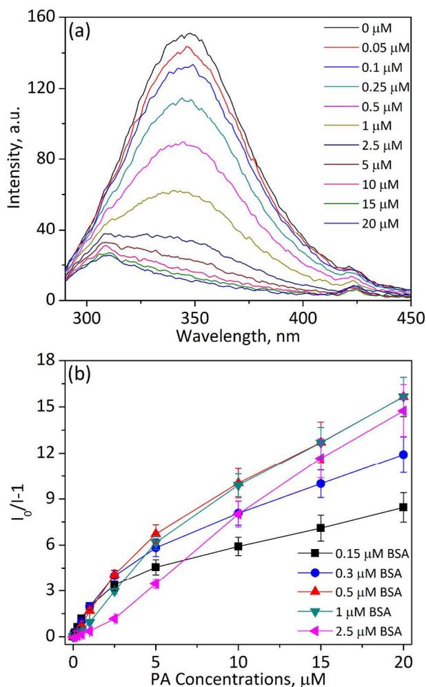
**Fig. 1** (a) Fluorescence spectra of 0.5  $\mu\text{M}$  BSA upon addition of various PA concentrations in water. (b) Stern-Volmer Plots for PA detection using various concentrations of BSA.
