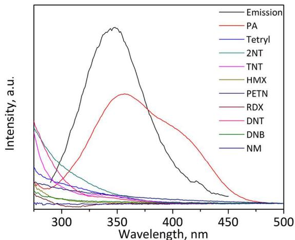
**Fig. 3** Absorption spectra of various explosive analytes and emission spectrum of BSA in aqueous solutions.
