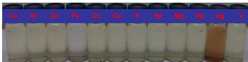
Fig. 2 Photographic image of L (20 \mu M) in the presence of different metal ions
