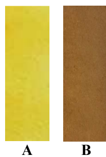
Fig. 7 Photographs of the filter paper coated with L used for the detection of \text{Ag}^+ . (a) Filter paper coated with L ( 20 \mu\text{M} ), (b) Probe L test kit immersed in \text{Ag}^+ solution.
