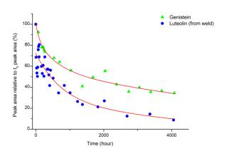
Figure 6: The photo-degradation rates of genistein (2) and luteolin (1).
