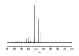
**Figure 4:** MS/MS fragmentation of the  $[M - H]^-$  ion (m/z 283) of unknown component  $G_3$  under negative ion electrospray ionisation conditions (CE: 25 eV).
