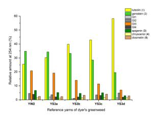
**Figure 5:** Relative amounts of the flavonoid dyes present in the acid-hydrolysed extracts of wool (YW2) and silk (YS3a) MODHT reference samples and a series of over-dyed (YS3b-d) samples; monitored at 254 nm.
