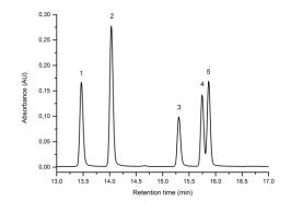
**Figure 1**: UPLC Method using PST BEH C18, 1.7  $\mu$ m, 2.1  $\times$  150 mm column, showing the separation of luteolin (1), genistein (2), apigenin (3), chrysoeriol (4) and diosmetin (5). Standard solution at 10  $\mu$ g mL<sup>-1</sup> recorded at 254 nm (5  $\mu$ L injection volume).
