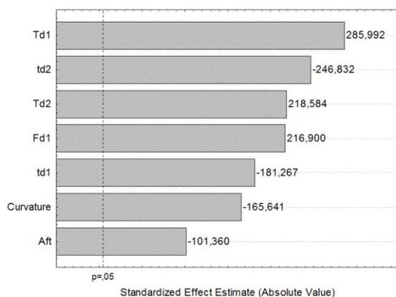
Figure 6 – Pareto chart of the effects of the factors evaluated in the thermal desorption of Tenax-TA, based on the  $2^{(6-2)}$  design
