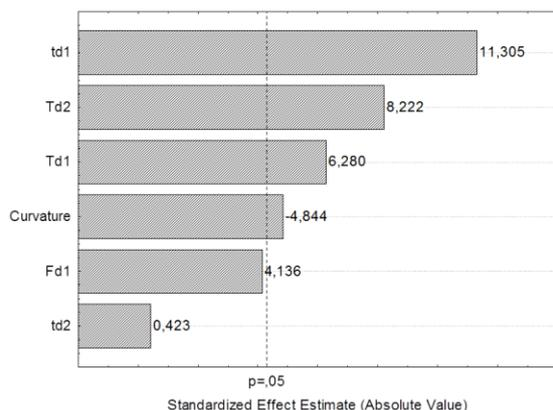
Figure 9 – Pareto chart of the effects of the factors on the thermal desorption of the TA-CX-CS adsorbent, based on the  $2^{(5-2)}$  design
