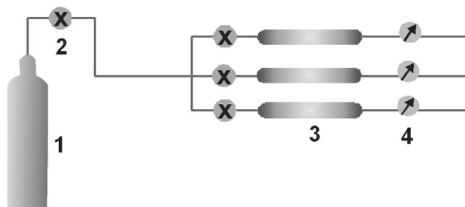
**Figure 1** – Preconcentration system for organic contaminants in VCM: (1) steel cylinder containing pressurized VCM; (2) flow control valve; (3) adsorbent tubes; (4) flow meter
