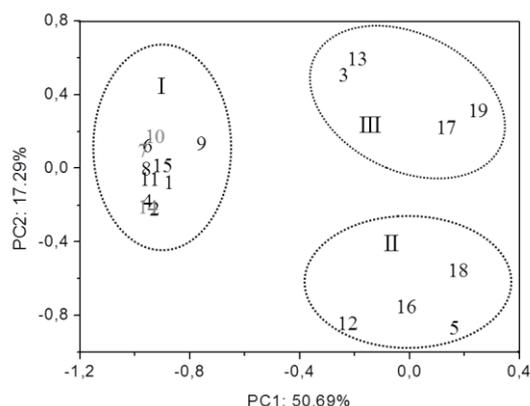
Figure 14 – Principal components analysis (PC1 x PC2) of VCM contaminants identified at the different points of the process. (1) 1,3-Butadiene, (2) Benzene, (3) 2,4-Hexadiene, (4) Toluene, (5) 1-Octanol, (6) Ethylbenzene, (7) o-Xylene, (8) p-Xylene, (9) Styrene, (10) Propylbenzene, (11) 1,4-Dichlorobenzene, (12) Chloroacetophenone, (13) Propenylbenzene, (14) Phenol, (15) Acetophenone, (16) Naphtalene, (17) Benzaldehyde, (18) 1,2-Dichloroethane, (19) Trichloromethane.
