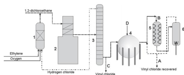
Figure 11 – Simplified diagram of the stages of the production, storage and recovery process of vinyl chloride monomer and of the sample collection points. (1) ethylene oxychlorination reactor; (2) 1,2-DCE pyrolysis furnace; (3) distillation tower which separates HCl and VCM; (4) VCM spherical storage tank; (5) VCM polymerization reactor; (6) PVC purification post-reactor; (A) unreacted recovered VCM; (B) VCM from the spherical tank + recovered VCM; (C) fresh VCM; (D) VCM from the spherical tank
