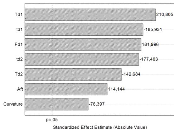
Figure 8 – Pareto chart of the effects of the factors on the thermal desorption of the TA-CX-CS adsorbent, based on the  $2^{(6-2)}$  design
