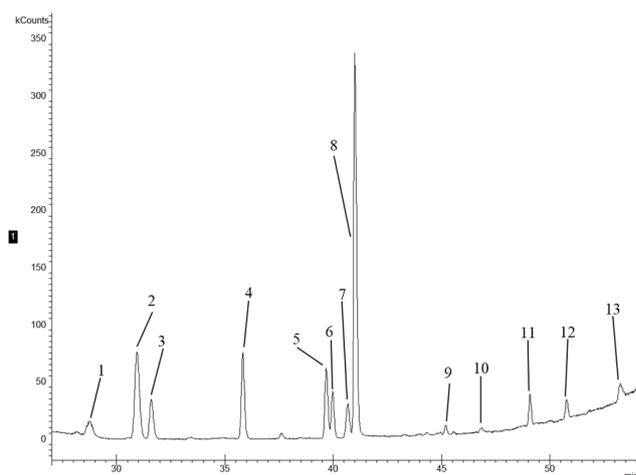
Figure 10 – Characteristic GC-MS chromatogram of a VCM sample from point D (spherical tank). Contaminants were preconcentrated on Tenax-TA ( $20 \text{ mL min}^{-1}$  flow rate and 1.5 L final sample volume) and desorbed according to conditions on Table 4.
