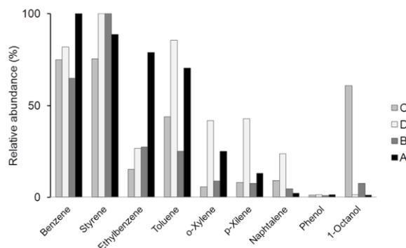
Figure 12 – Relative abundances of the VCM contaminants as a function of the sampling point. A- recovered VCM; B- VCM at the polymerization reactor inlet; C- VCM at the distillation tower outlet; D- VCM in the spherical tank
