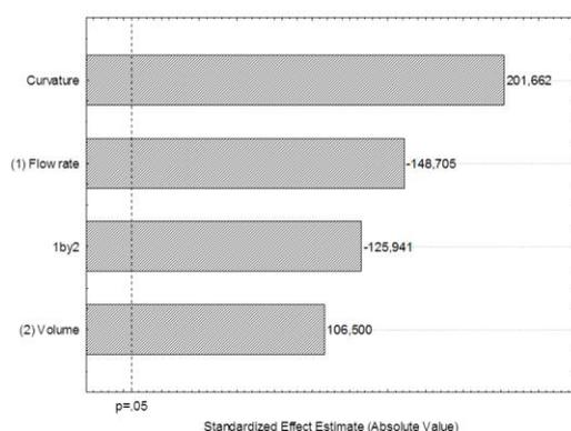
Figure 3 – Pareto chart of the factors flow, volume and flow/volume interaction, for adsorption preconcentration on Tenax-TA/Carboxen1000/CarbosieveSIII
