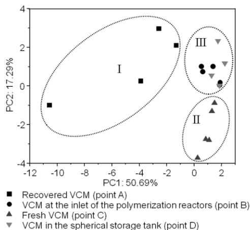
Figure 13 – Principal components analysis (PC1 x PC2) of VCM samples collected at different points of the process
