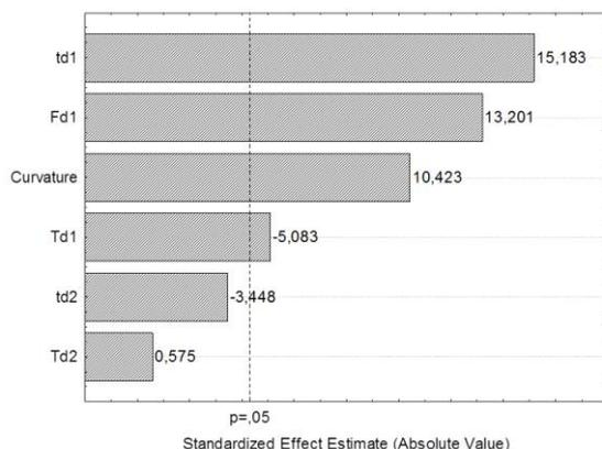
Figure 7 – Pareto chart of the effects of the factors for the thermal desorption of Tenax-TA, based on the  $2^{(5-2)}$  design
