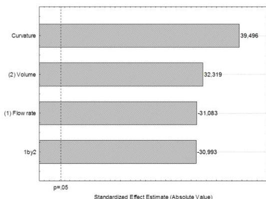
Figure 2 – Pareto chart of the factors flow, volume and flow/volume interaction, for adsorption preconcentration on Tenax-TA
