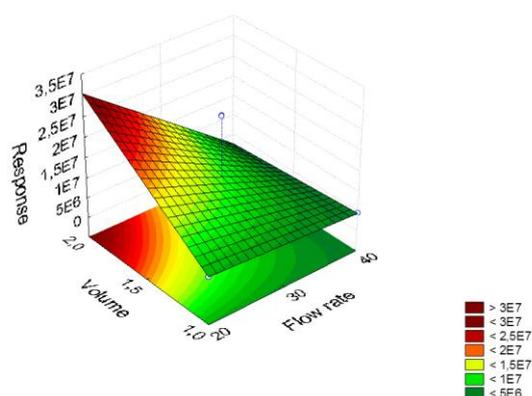
Figure 5 – Response surface of adsorption on Tenax-TA/Carboxen1000/CarbosieveSIII
