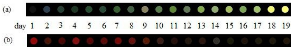
Fig. 7 The color changes of bromocresol green (a) and neutral red (b) during 19 days
