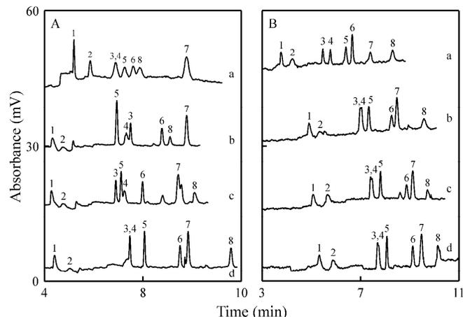
**Fig. 3** (A) Electropherograms showing the impact of SDS in 0.100% PEO solutions: SDS of (a) 0 mM, (b) 20 mM, (c) 30 mM, and (d) 50 mM. (B) Effect of the PEO concentration on the stacking and separation of the analytes: PEO solutions of (a) 0%, (b) 0.050%, (c) 0.075%, and (d) 0.125% were prepared in 15 mM tetraborate buffer containing 40 mM SDS. Other conditions were same as those in Fig. 2B.
