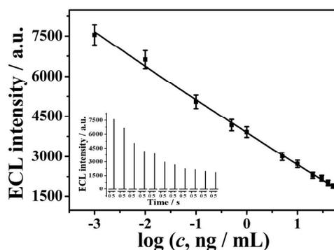
**Fig. 4** Calibration curve of the immunosensor to different concentration of OTA. Error bar = RSD,  $n = 3$ .
