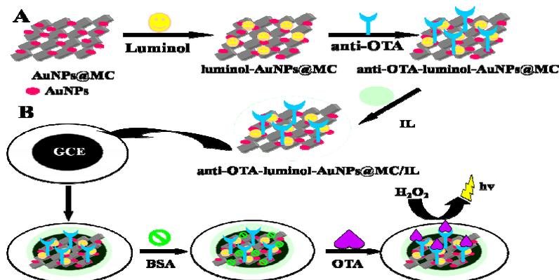
**Fig. 1.** (A) Fabrication process of anti-OTA-luminol-AuNPs@MC/IL and (B) Schematic diagram of the fabrication of the immunosensor.
