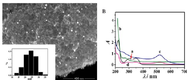
**Fig. 2** SEM (A) image of Au@MC (inset was the image of size distribution of Au NPs) and UV-vis (B) absorption spectra of luminol (a), anti-OTA (b), Au NPs (c) and anti-AFB<sub>1</sub>-luminol-Ag@MC (d).
