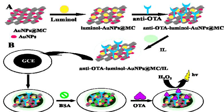
Ultrasensitive electrochemiluminescence immunosensor for detection of ochratoxin A based on gold nanoparticles hybridized mesoporous carbon
