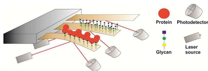
Fig. 4: Detection of glycan-protein interactions with microcantilever arrays.
