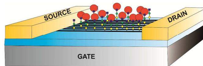
**Fig. 3:** CNT-based FET device for monitoring of glycan-protein interactions.
