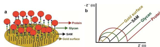
**Fig. 2:** Scheme of operation of EIS-based glycan biosensor, (a) the structure of an active biosensor surface, (b) a Nyquist plot applied for data analysis.
