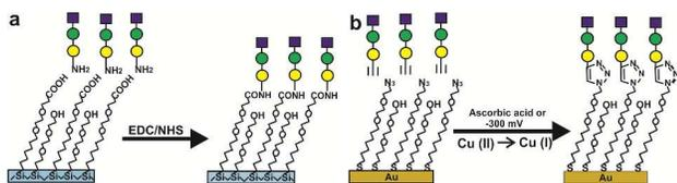
**Fig. 1:** Immobilization of derivatized glycans onto a functionalized biosensor surface. (a) Glycan immobilization onto silanized surface *via* EDC/NHS (amine coupling) and (b) copper catalyzed azid-alkyne cycloaddition (click chemistry) onto thiolated SAM on a gold surface.
