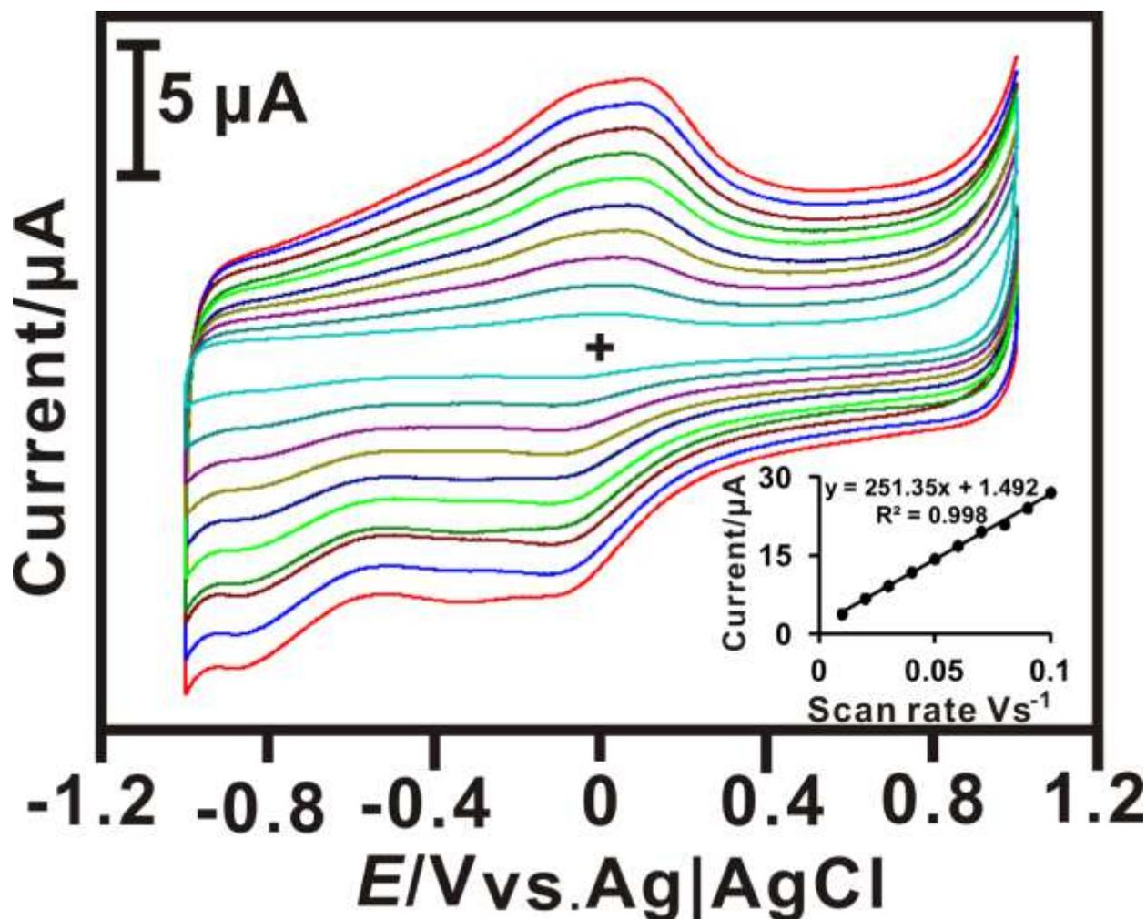
Fig.2. Different scan rate studies of the GCE/MWCNTs/ZrO<sub>2</sub> modified electrode in pH 7 at scan rate varies from 0.01 to 0.1 V/S. Inset shows a current vs. scan rate plot at pH7.
