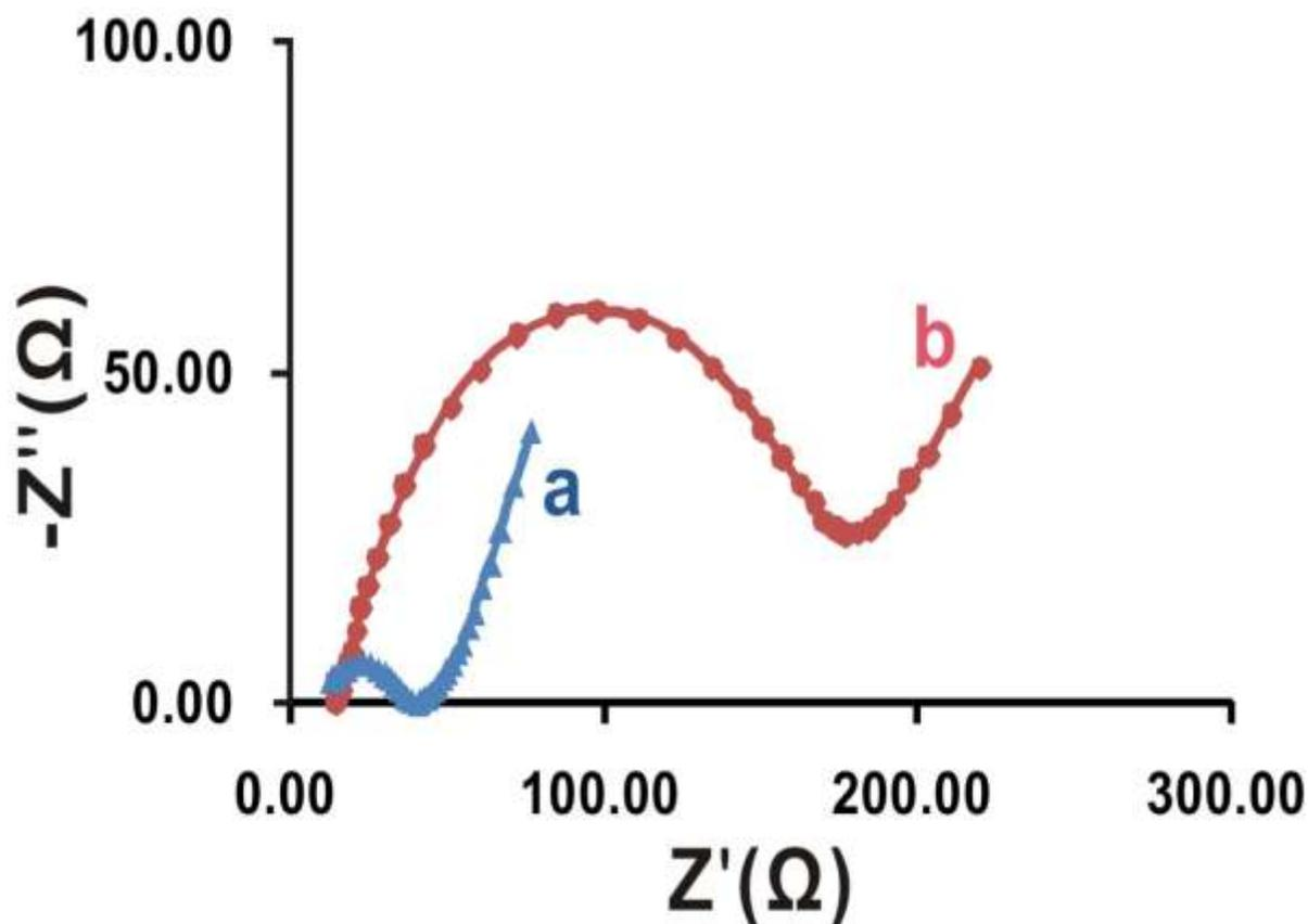
Fig.3. EIS of a) GCE/*f*MWCNTs /ZrO<sub>2</sub> and b) bare GCE in 5mM [Fe (CN)<sub>6</sub>]<sup>3-/4-</sup> in pH7 PBS.
