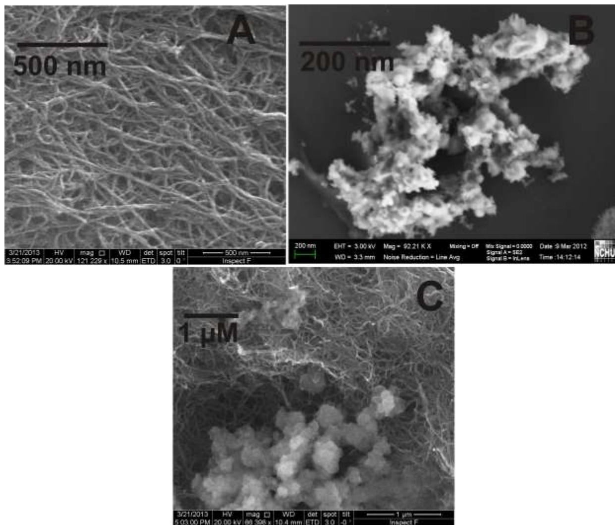
**Fig.5.FESEM images of (A) *fMWCNTs*, (B)  $ZrO_2$  and (C) *fMWCNTs/ZrO\_2* films at different magnifications.**
