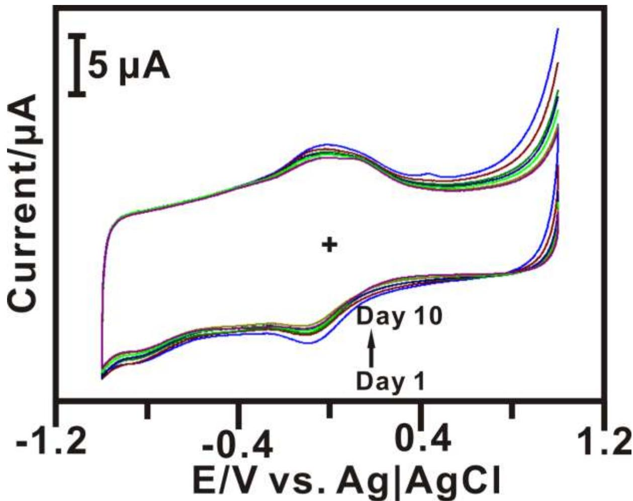
Fig.8. CV response of *f*MWCNTs/ZrO<sub>2</sub> nanocomposite film modified GCE in the pH 7 PBS for 10 days (a-g).
