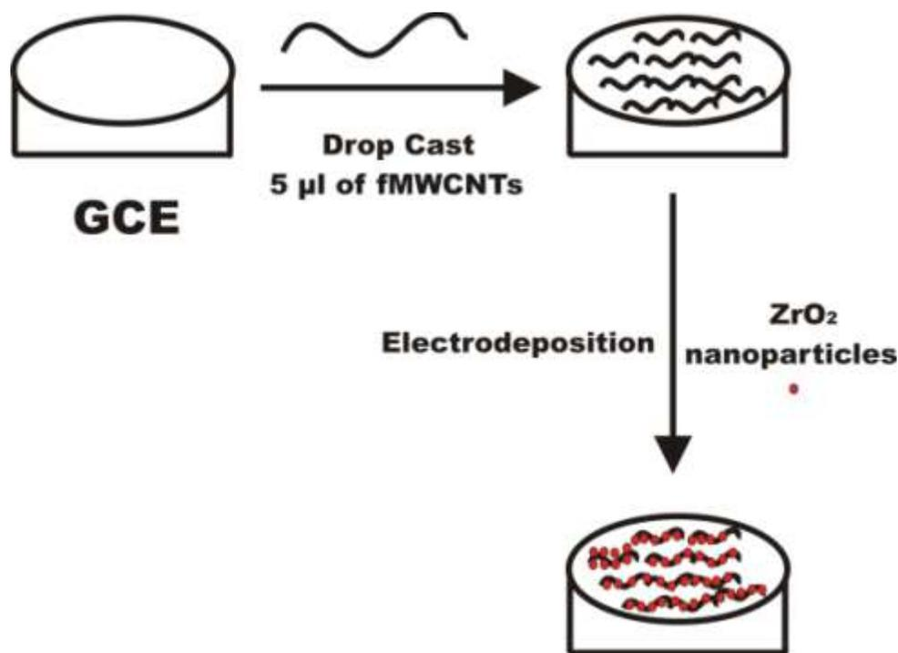
**Scheme 1.** Schematic representation of single step fabrication of *f*MWCNTs/ZrO<sub>2</sub> nanocomposite modified electrode.
