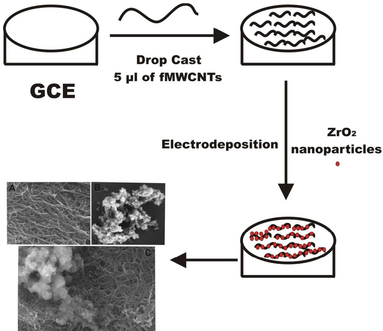
Electrochemical fabrication of fMWCNTs/ZrO<sub>2</sub> nanocomposite film on the glassy carbon electrode electrode surface.
