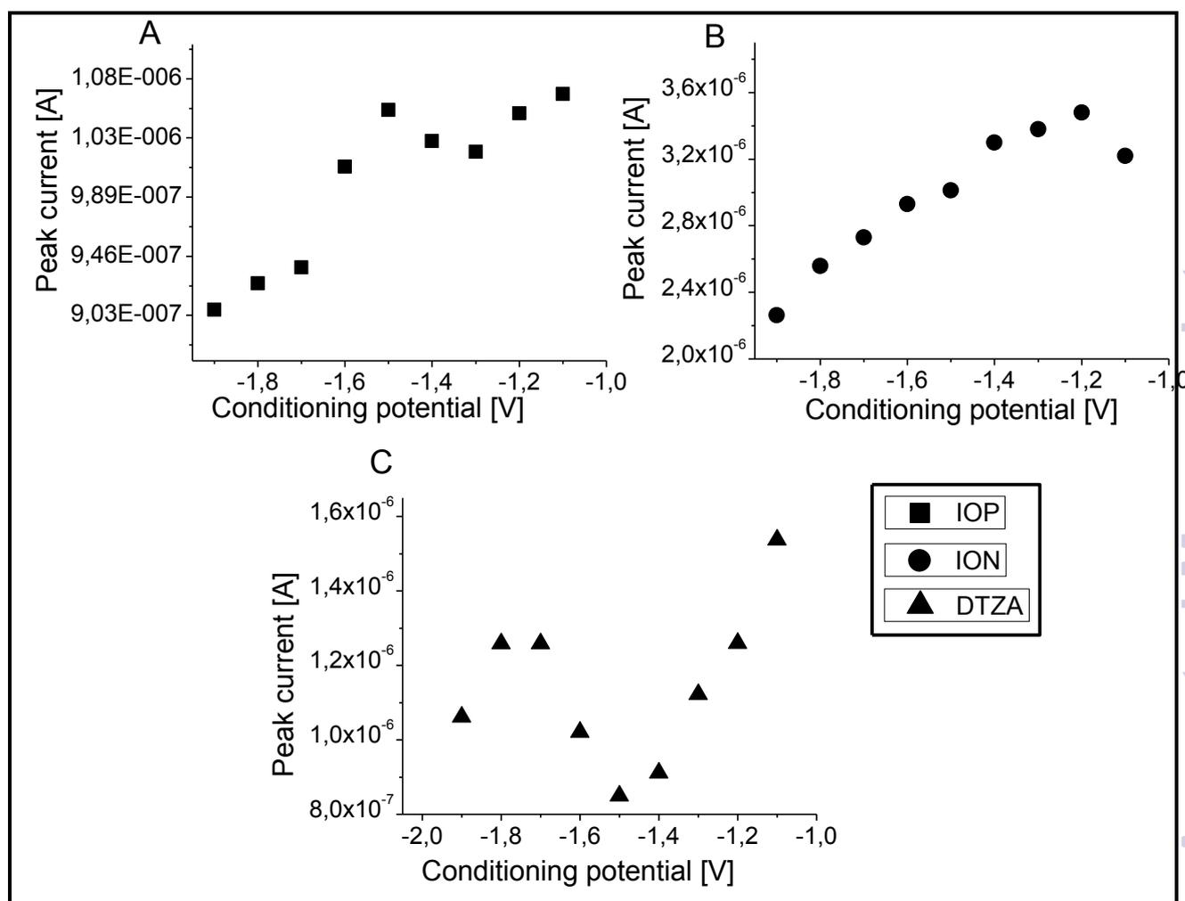
**Fig. 6** Plot of oxidative peak current response versus conditioning potential of  $3.9 \times 10^{-5}$  M IOP (A),  $6.0 \times 10^{-6}$  M of ION (B),  $4.0 \times 10^{-6}$  M of DTZA (C) at GCE (vs. Ag|AgCl||KCl<sub>(sat)</sub>).
