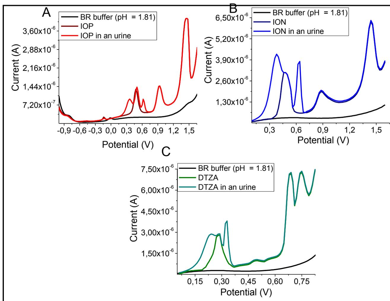
**Fig. 8** DPV voltammograms of ION (A), IOP (B) and DTZA (C) in BR buffer (pH = 1.81) of artificial urine samples after SPE procedure at GCE (vs.  $\text{Ag}|\text{AgCl}||\text{KCl}_{(\text{sat})}$ ).
