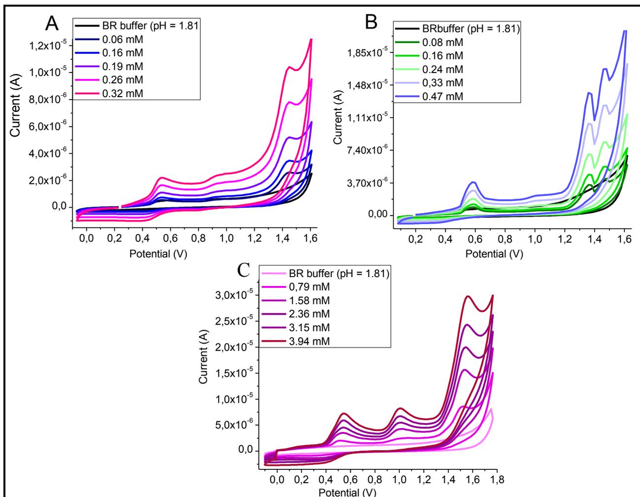
**Fig. 2** Cyclic voltammograms recorded for determination of ION (A), DTZA (B) and IOP (C) in mixture of BR buffer at pH 1.81/methanol (9/1, v/v) at GCE (vs. Ag|AgCl||KCl<sub>(sat)</sub>).
