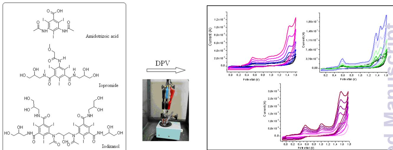
This manuscript shows the ability to quickly detect the concentration of three iodinated X-ray contrast agents (iopromide, iodixanol and amidotrizoic acid) using differential pulse voltammetry method.
