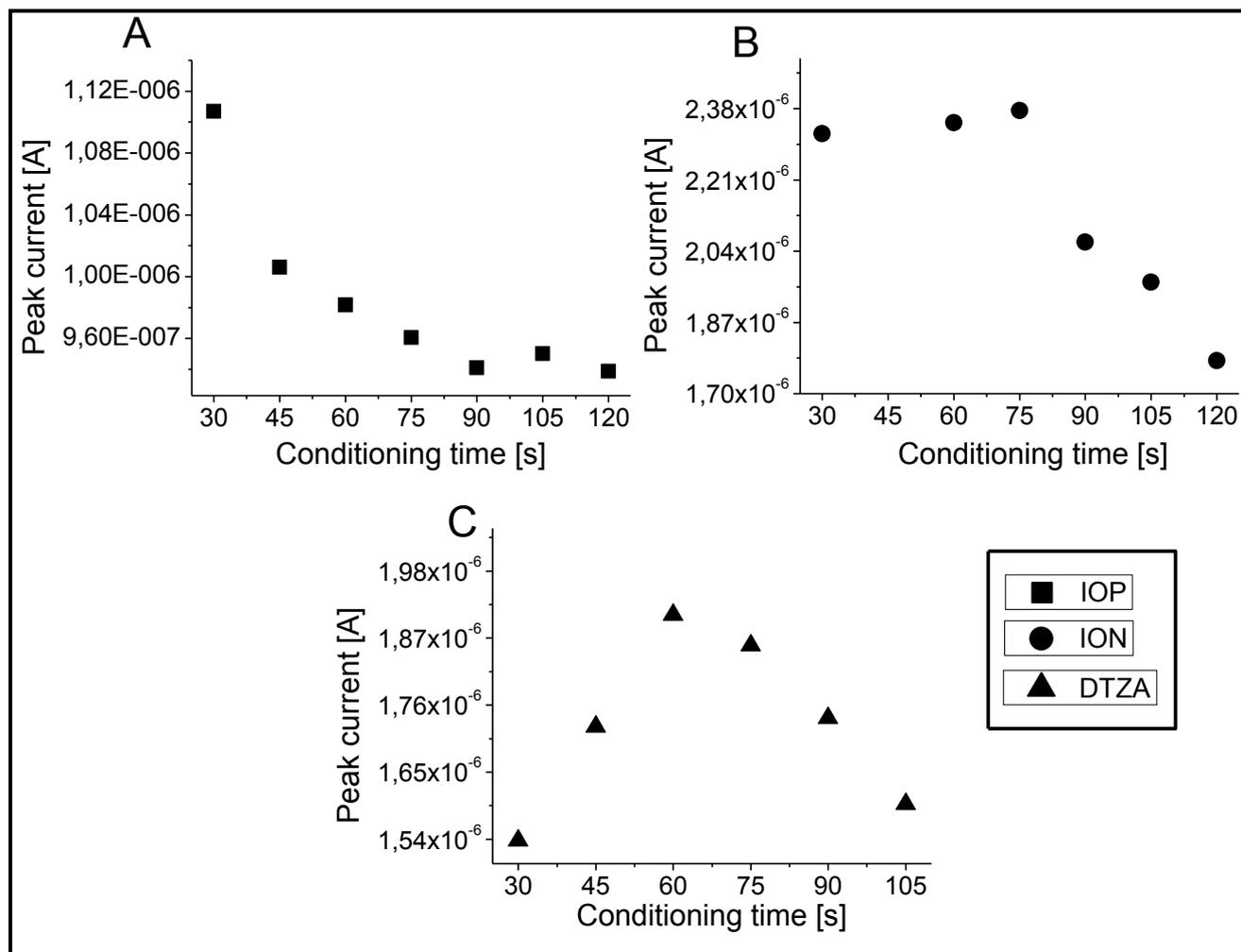
**Fig. 7** Plot of oxidative peak current response versus conditioning time of  $3.9 \times 10^{-5}$  M IOP (A),  $6.0 \times 10^{-6}$  M of ION (B),  $4.0 \times 10^{-6}$  M of DTZA (C) in BR buffer (pH = 1.81) at GCE (vs. Ag|AgCl||KCl<sub>(sat)</sub>).
