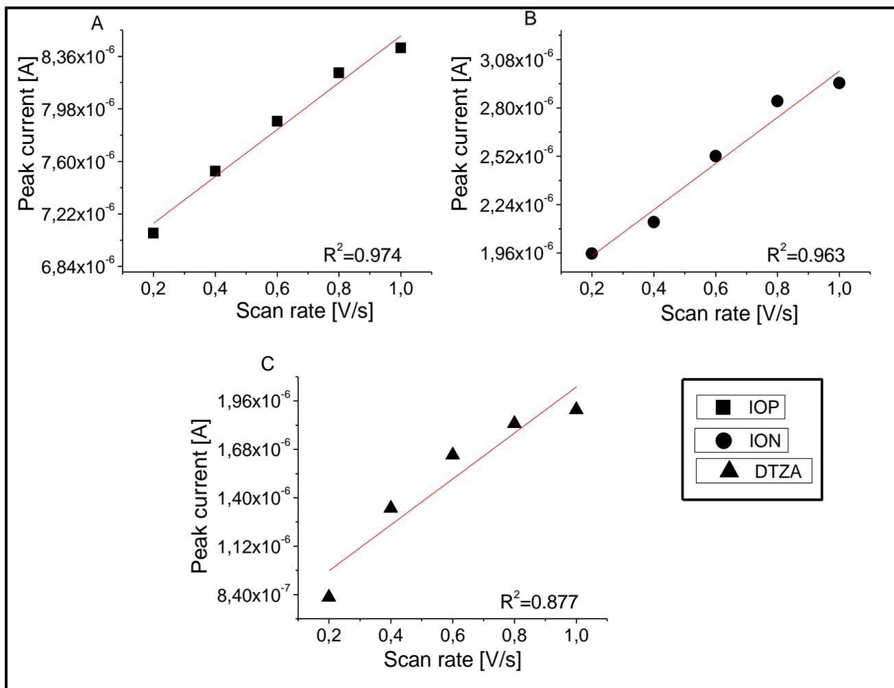
**Fig. 5** Plot of oxidative peak current versus potential scan rate of  $1.18 \times 10^{-4}$  M of IOP (A),  $0.6 \times 10^{-4}$  M of ION (B) and  $0.8 \times 10^{-5}$  M of DTZA (C) in BR buffer (pH = 1.81) at GCE (vs. Ag|AgCl||KCl<sub>(sat)</sub>).
