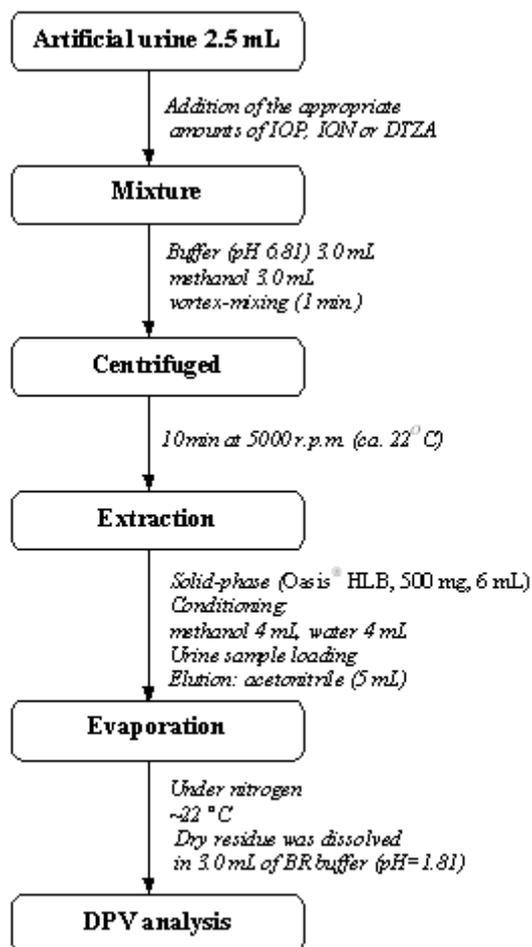
**Fig. 1** Procedure of artificial urine samples preparation for determination of the IOP, ION and DTZA.
