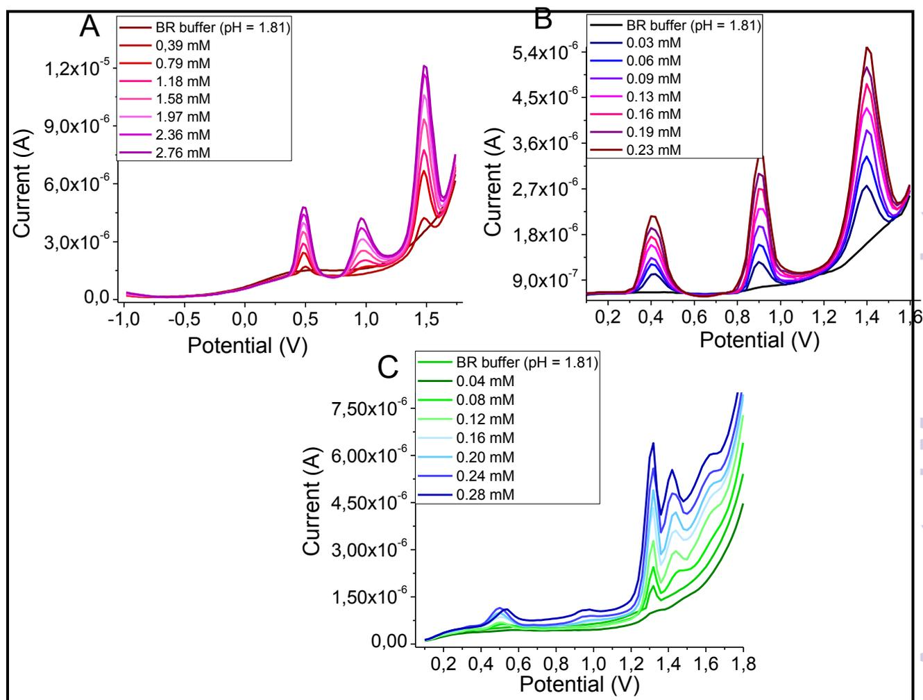
**Fig. 3** DPV voltammograms recorded for determination of ION (A), IOP (B) and DTZA (C) in mixture of BR buffer at pH 1.81/methanol (9/1, v/v) at GCE (vs. Ag|AgCl||KCl<sub>(sat)</sub>).
