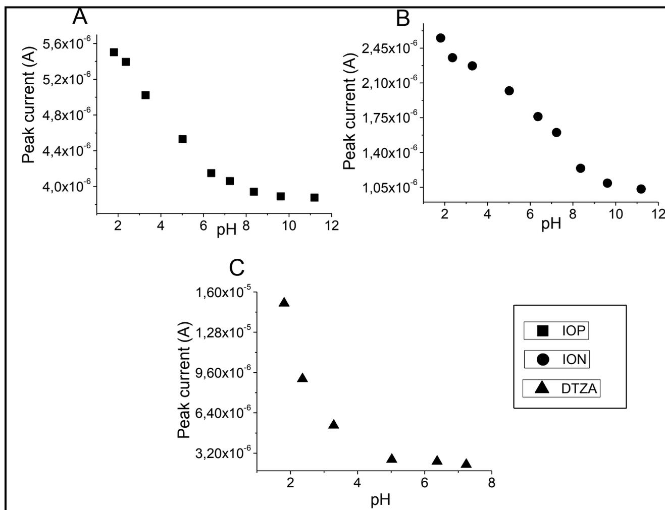
**Fig. 4** Plot of oxidative peak current response versus pH of BR buffer containing  $3.9 \times 10^{-5}$  M IOP (A),  $6.0 \times 10^{-6}$  M of ION (B),  $4.0 \times 10^{-6}$  M of DTZA (C) at GCE (vs.  $\text{Ag}|\text{AgCl}||\text{KCl}_{(\text{sat})}$ ).
