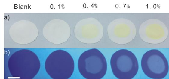
**Fig. 6** Colorimetric and fluorescent visualization of FDA-coated organic membrane after exposure to different concentrations of hydrazine (0.1%, 0.4%, 0.7% and 1.0%) by naked-eye under the sunlight (a) and UV light of 365 nm (b), respectively. The scale bar is 1.0 cm.
