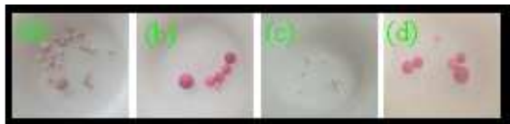
Fig. 15 (a) Bead 2 ; (b) 2 + \text{Hg}^{2+} (300 \mu\text{L} ); (c) 2 + all metal salts (300 \mu\text{L} each metal salt) except \text{Hg}^{2+} ; (d) 2 + all metal salts (300 \mu\text{L} of each metal salt) + \text{Hg}^{2+} (300 \mu\text{L} ); (concentration of all metal salts: 5.2 \times 10^{-4} M).
