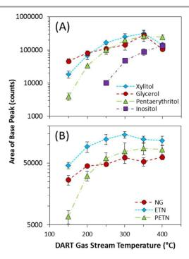
Figure 5 Effect of DART gas stream temperature on select sugar alcohols (A) and nitrate ester explosives (B). In both instances the data points represent the average peak area obtained by integrating the total area under the extracted ion chromatogram of the base peak ([M-H] for sugar alcohols and [M+NO<sub>3</sub>] for nitrate ester explosives). Uncertainty is expressed as the standard deviation of four replicate samples.
