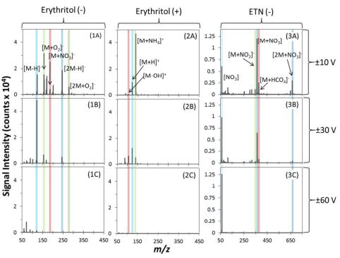
Figure 2 Representative mass spectra of erythritol in negative mode (1) and positive mode (2) as well as ETN in negative mode (3) at ±10 V (A), ±30 V (B), and ±60 V (C) orifice 1 plate voltages. Major peaks for each spectrum are highlighted.
