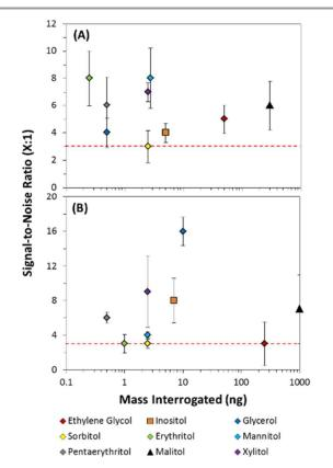
Figure 3 Measured sensitivities and average signal-to-noise ratios (S/N) for sugar alcohols in both negative (A) and positive (B) ionization mode. Error bars represent the standard deviation in the S/N measurement across 4 measurements. The dotted red line indicates the threshold of 3:1 S/N.
