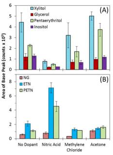
Figure 6 Response of representative sugar alcohols (A) and nitrate ester explosives (B) in the presence of select dopants. The peak area represents the area of the base peak ([M-H] for sugar alcohols and [M+NO<sub>3</sub>] for nitrate ester explosives) from the extracted ion chromatogram. Uncertainty is expressed as the standard deviation of four replicate samples.
