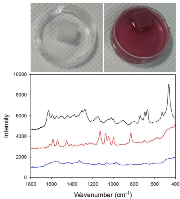
**Fig. 2** Transmission Raman spectra of AuNP-incorporated PE I (red), PE II (black), and melamine sponges (blue). The spectra are offset for clarity. Pictures on the top show cubes of the melamine sponge in a Petri dish before (left) and after (right) being soaked with the AuNP solution.
