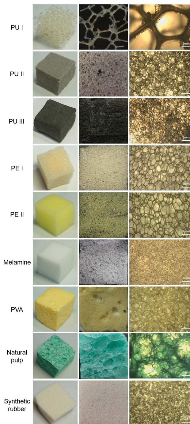
**Fig. 1** (a) The images of nine different sponges evaluated for use as a TSERS substrate. The images in the first, second, and third columns show the actual appearances of the sponges (volume: approximately 2.0 - 2.5 cm<sup>3</sup>), top-view images (~1.0 × 1.0 cm<sup>2</sup>) of thin-sliced sponges, and the corresponding enlarged images with 40-fold magnification, respectively.
