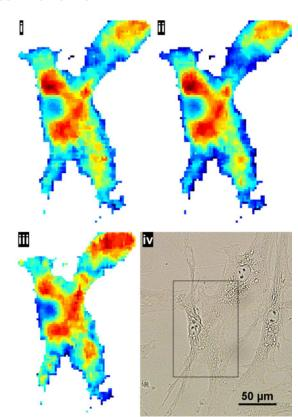
Fig. 8: Example image from a targeted region of cultured human skin fibroblasts measuring  $^{\circ}90 \times 50~\mu m$ ; Comparing vector normalised, integrated lipid region chemimap (2800-3000 cm $^{-1}$ ) before (i) and after noise reduction (ii) versus the image once the data has been noise-reduced, RMieS-EMSC corrected then vector normalised (iii). The optical image was acquired with a 20× objective, at a pixel resolution of 0.53  $\mu m$  (iv).
