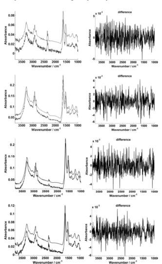
Fig. 5: Typical single pixel spectra illustrating the PCA-based noise reduction algorithm using 50 retained PCS. The high-magnification image representative spectra A-D are shown before and after noise reduction respectively (left). The differences between the raw and corrected spectrum in each case area also displayed (right).
