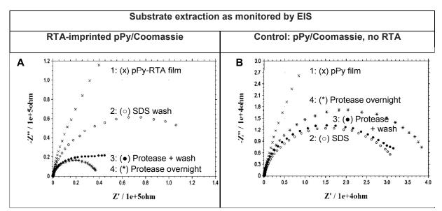
**Figure 2. Substrate removal from MICP film. (A):** MICP pPy/Coomassie film imprinted with RTA; **(B)** same without RTA. (A&B): 1: after pPy polymerization by CV; 2: after 1h wash PBS/ 0.5% SDS; 3: after protease treatment 2h and repeated PBS/SDS wash; 4: after protease treatment overnight.
