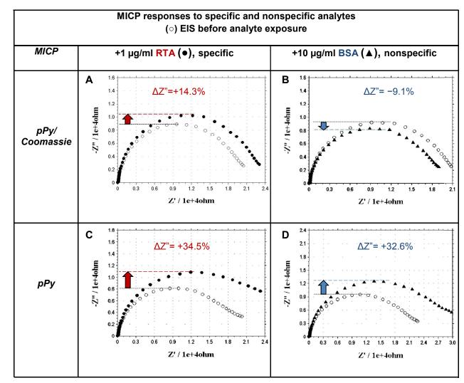
**Figure 3**. **Macromolecular dopant is needed for specificity of MICP.** Impedance changes in RTAimprinted pPy/Coomassie MICP (**A&B**) and in pPy MICP (**C&D**) upon interaction with specific analyte (●): 1 μg/ml RTA, **A&C**; and nonspecific analyte (▲): 10 μg/ml BSA, **B&D**. (○): EIS spectra before incubation.
