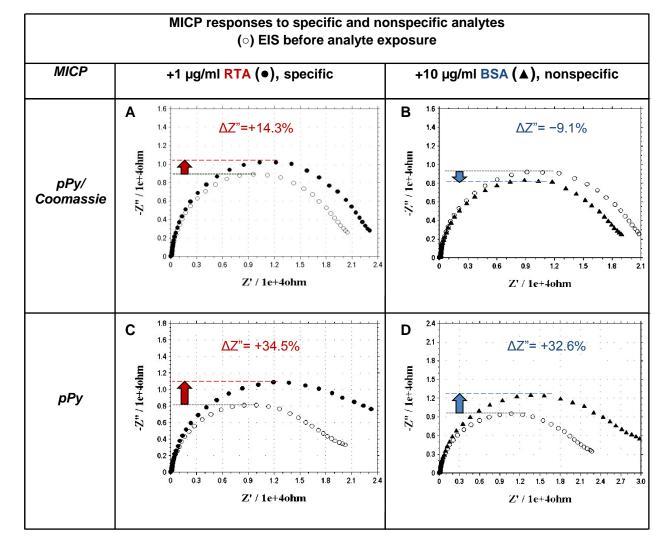
Figure 3. Macromolecular dopant is needed for specificity of MICP. Impedance changes in RTAimprinted pPy/Coomassie MICP (A&B) and in pPy MICP (C&D) upon interaction with specific analyte ( $\bullet$ ): 1 µg/ml RTA, A&C; and nonspecific analyte ( $\blacktriangle$ ): 10 µg/ml BSA, B&D. ( $\circ$ ): EIS spectra before incubation.
