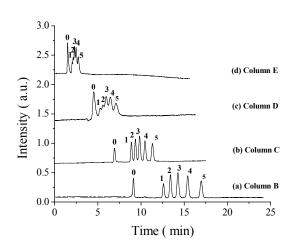
Fig. 3 Effect of the ratio of POSS-MA/BMAB on separation of ABs on POSS-BMAB hybrid monoliths. Conditions: mobile phase, ACN/H<sub>2</sub>O (75/25, v/v); flow rate, 0.05 mL/min; detection wavelength, 214 nm; POSS–BMAB monoliths: 52 cm  $\times$ 75  $\mu$ m i.d. (30 cm effective length); supplement pressure, 1000 psi (a and b), 75psi (c and d). Solutes 0, thiourea; 1, benzene; 2, toluene; 3, ethylbenzene; 4, propylbenzene; 5, butylbenzene.
