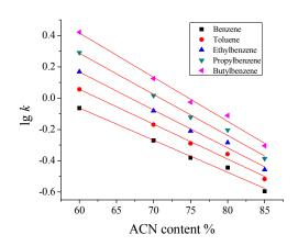
Fig. 9 The effect of ACN content in mobile phase on the retention factor  $\lg k$  of ABs on Clumn B. Conditions are same as in Fig.3
