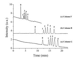
25 Fig. 4 Effect of thiol-ene click reaction temperature on separation of ABs on POSS-BMAB hybrid monolith. Conditions: supplement pressure, 1000 psi (a, b), 75psi (c). Other conditions are same as in Fig. 3
