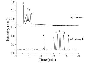
Fig. 5 Effect of the ratio of toluene-dodecanol on separation of ABs on 30 POSS-BMAB monoliths. Conditions: supplement pressure, 1000 psi (a), 100psi (b). Other conditions are same as in Fig. 3
