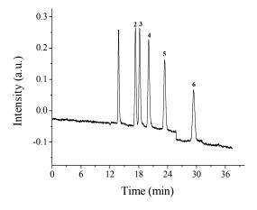
Fig. 12 Separations of anilines on the column B in cLC. Conditions: mobile phase, ACN/H<sub>2</sub>O (65/35, v/v). Other conditions are same as in Fig. 5. Solutes 1, o-phenylenediamine; 2, aniline; 3, p-toluidine; 4, 25 benzidine; 5, 2,4-dinitroaniline; 6, 1-aminonaphthalene.
