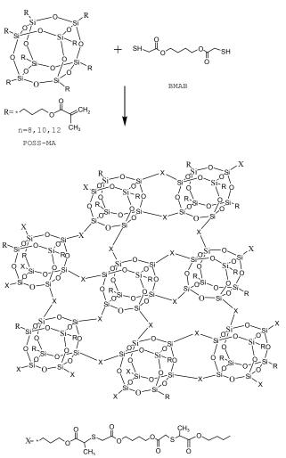
Fig.1 Preparation of the hybrid monoliths via thiol-ene click reaction of POSS-MA with BMAB
