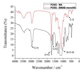
Fig. 6 FT-IR spectra of POSS-MA and POSS-BMAB hybrid monolith (Column B).
