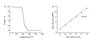
Fig. 7 TGA of POSS-BMAB hybrid monolith at a heating rate of 10°C /min in air (a) and the relationships between flow rate and the back pressure drop of POSS-BMAB hybrid monolith (b)
