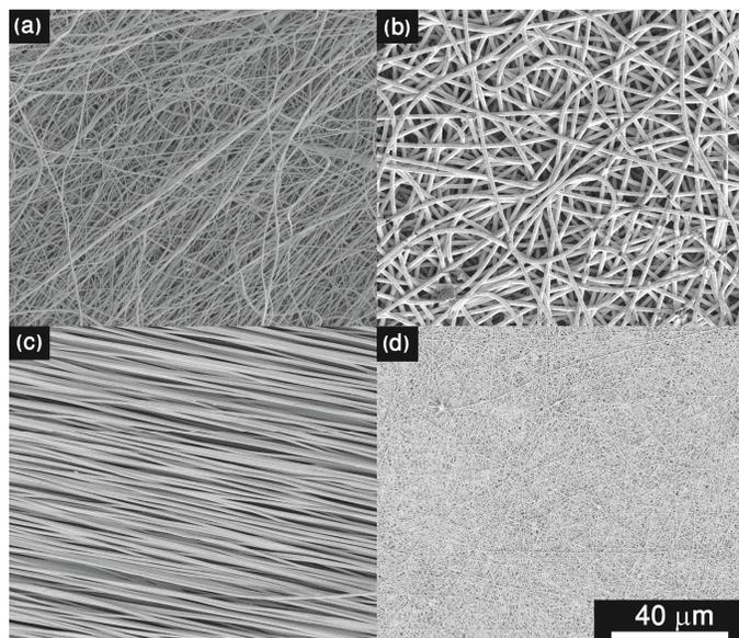
**Fig. 1.** SEM images of the polymer mats covered with 90 nm of gold, working as SERS platforms. We have tested four polymer mats: (a) PVDF, (b) PLLA-a, (c) PLLA-b and (d) nylon. The PLLA-a is a nonwoven mat, whereas PLLA-b is a woven mat. We present additional SEM pictures in ESI.
