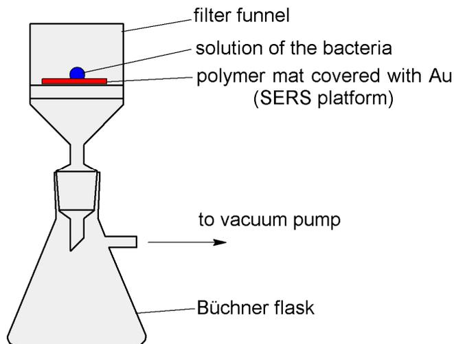
**Fig. 2** The scheme of embedding bacteria on the SERS platform directly from the solution. The vacuum pump generates partial vacuum which creates flow of liquid from the suspended droplet with bacterial cells. The spaces between the polymer fibers are small enough to keep bacterial cells on the surface of polymer mat, whereas the fluid pass through the polymer mat and filter funnel to the Büchner flask.
