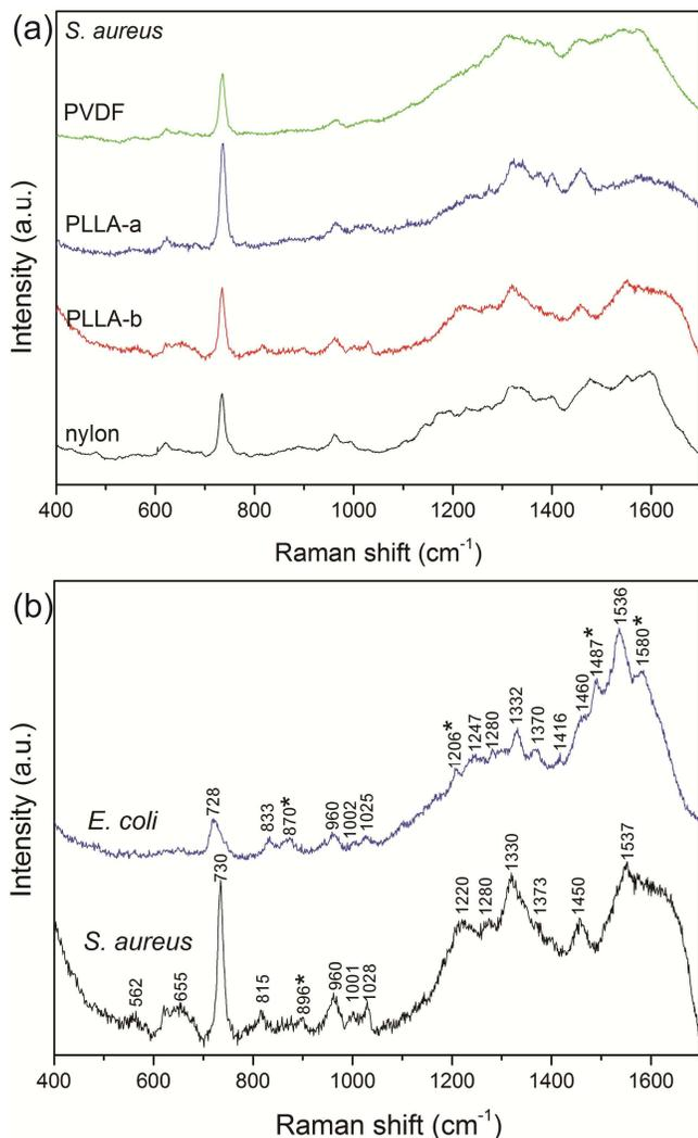
**Fig. 3** (a) SERS spectra of *S. aureus* recorded from four Au-coated polymer mats: PVDF, PLLA-a, PLLA-b and nylon. (b) Raman spectra of *E. coli* and *S. aureus* collected from Au-coated PLLA-b (woven) polymer mat. The bands marked with an asterisk (\*) were not assigned (they were not found in the literature). All the used polymer mats were covered with 90 nm of gold via PVD method.
