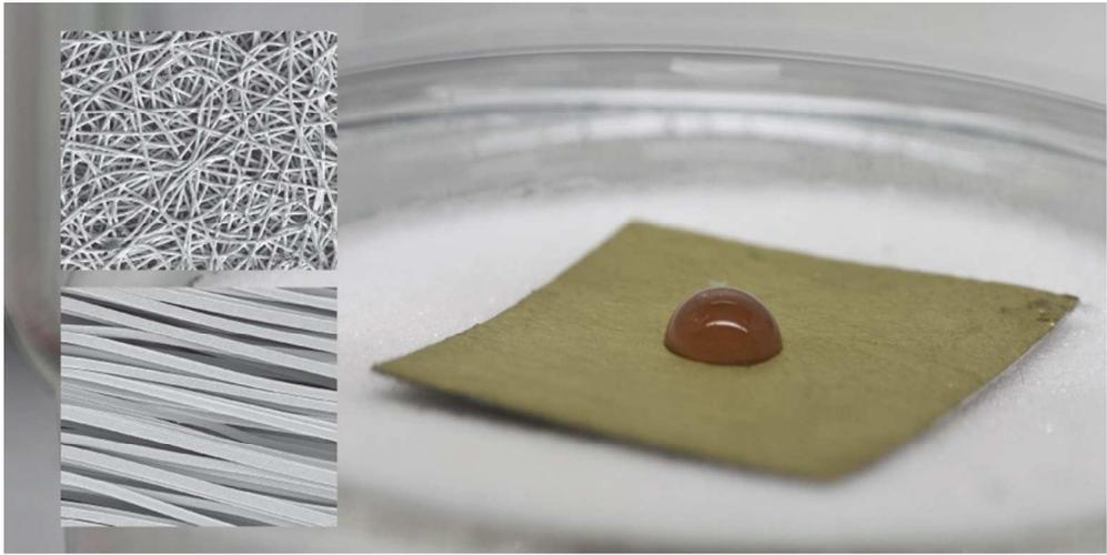
A new class of SERS substrates is presented that allows for simultaneous filtration of bacteria from any solution (blood, urine, water or milk), immobilization of bacteria on the SERS platform, and enhancing Raman signal of bacteria.
